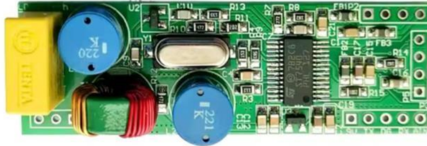
Figuer(4.H): Power Line Communication (PLC) Module
