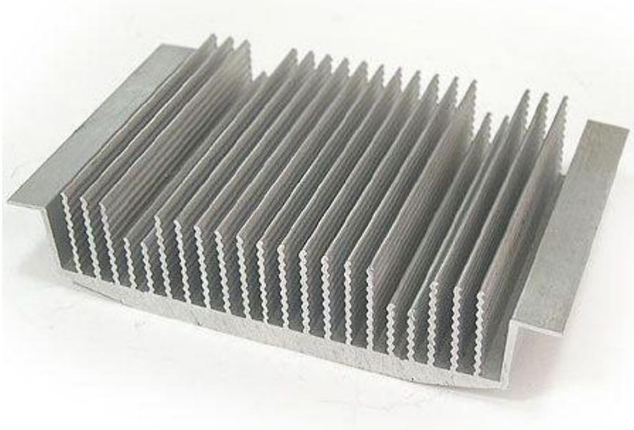
All semiconductor devices have electrical resistance, just like resistors and coils, etc. This means that when power diodes, transistors and MOSFETs power as heat energy will be dissipated. To save devices from thermal damaged, the heat must be removed at a fast enough rate to prevent excessive temperature rise.
