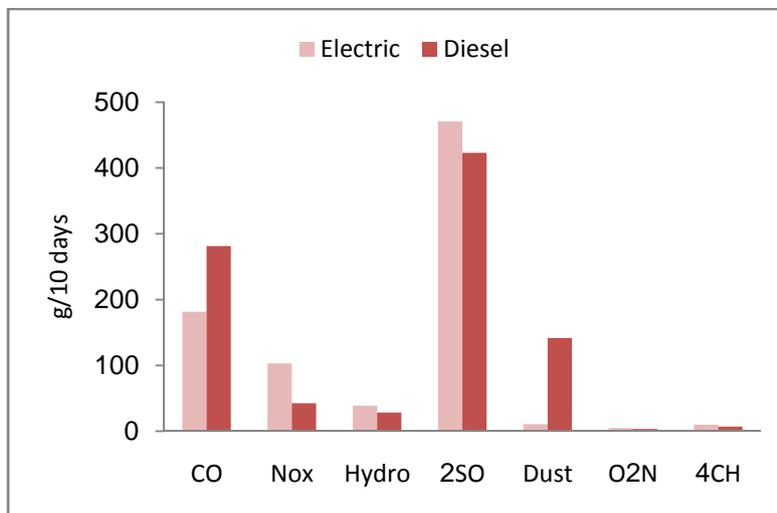
Fig.11: Different saved gas emissions by utilizing collective SWH of Birzeit university
