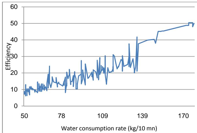
Fig.9: Collective SWH system effectiveness versus water consumption rate
