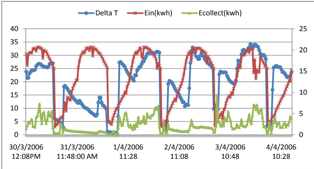
Fig.8b: Input solar energy and collector output energy with the corresponding temperature difference.
