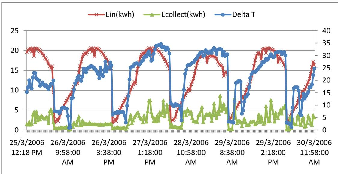
Fig.8-a: Input solar energy and collector output energy with the corresponding temperature difference. (25-30) May/2006
