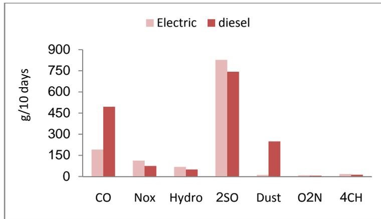
Fig.13: Different saved gas emissions by utilizing collective SWH Crown Plaza Hotel, Amman
