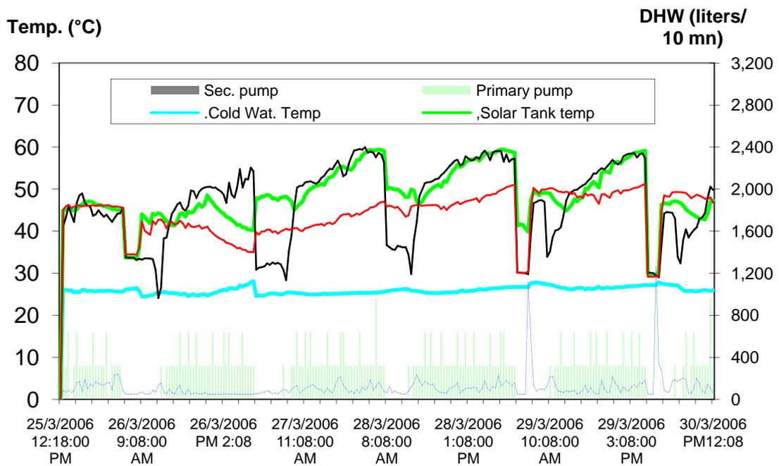
Fig.6-a: Temperature distribution in the SWH, solar radiation, and water flow consumption and primary pump work time from 25-30 March 2006.
