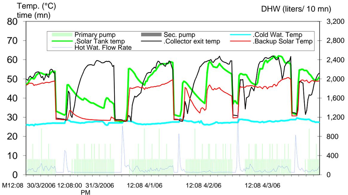
Fig.7-a: Temperature distribution in the SWH, solar radiation, and water flow consumption and primary pump work time from 30 March to 3 April 2006.
