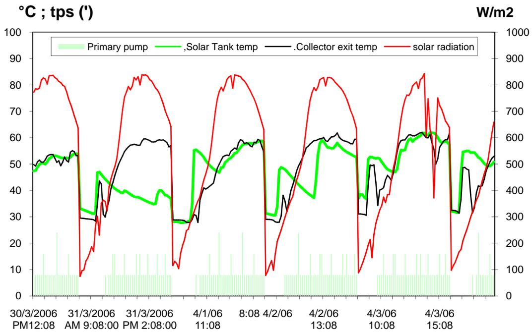
Fig.7-b: Solar tank and collector exit temperatures in the SWH and solar radiation from 30 March -3 April 2006.
