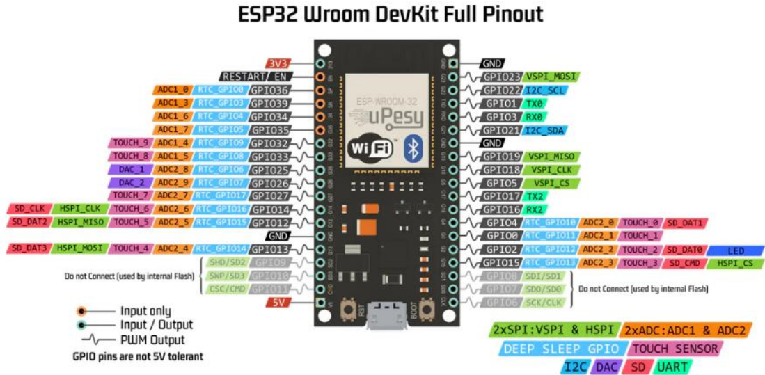
Pinout of an ESP32 board
