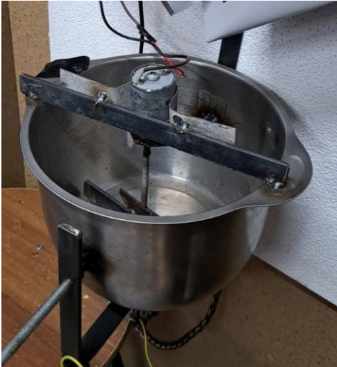
Figure 4 Mixing and Heating Unit
