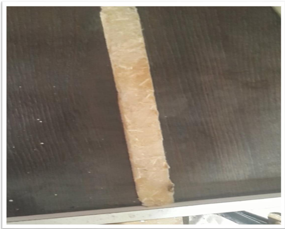
Figure 3.11: An epoxy blended with chicken feathers sample after 24 hours tensile strength by tensile machine.
