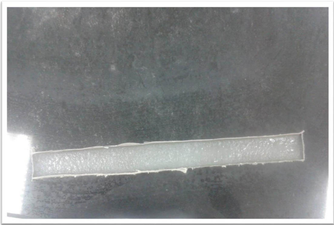
Figure 3.8: An epoxy sample before testing tensile strength by tensile machine.
