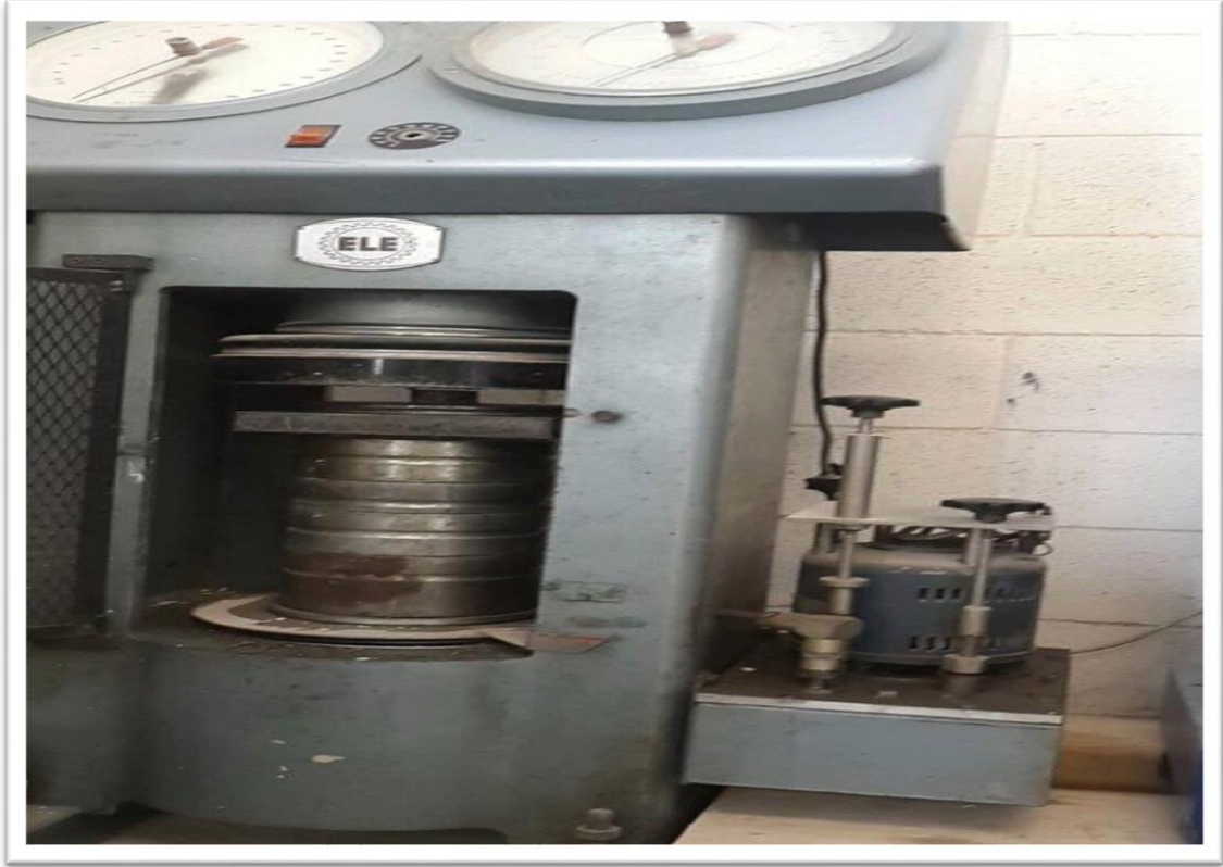
Figure 3.6: An epoxy with chicken feathers sample after 24 hours compression strength by compression machine.
