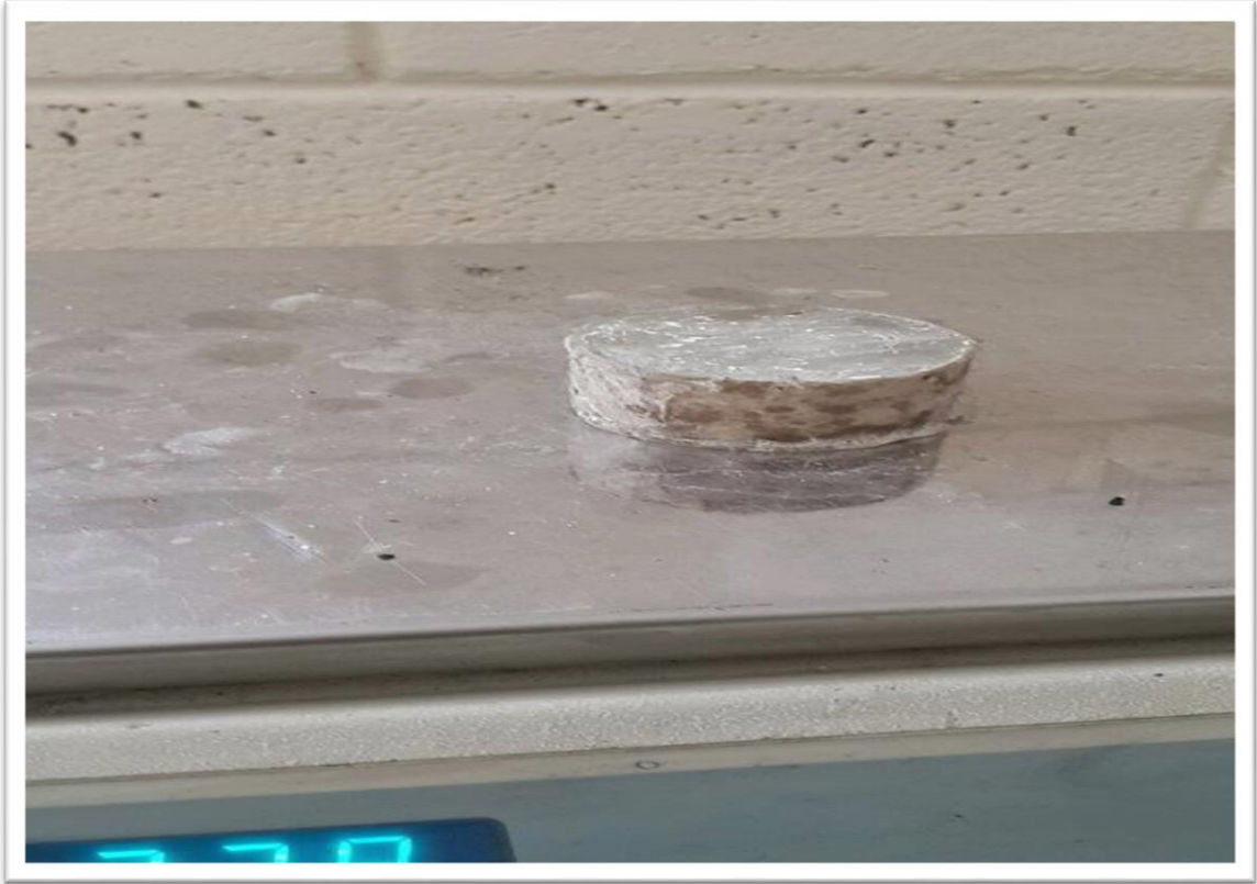
Figure 3.4: An epoxy sample in a cylinder after 24 hours compression strength by compression machine.
