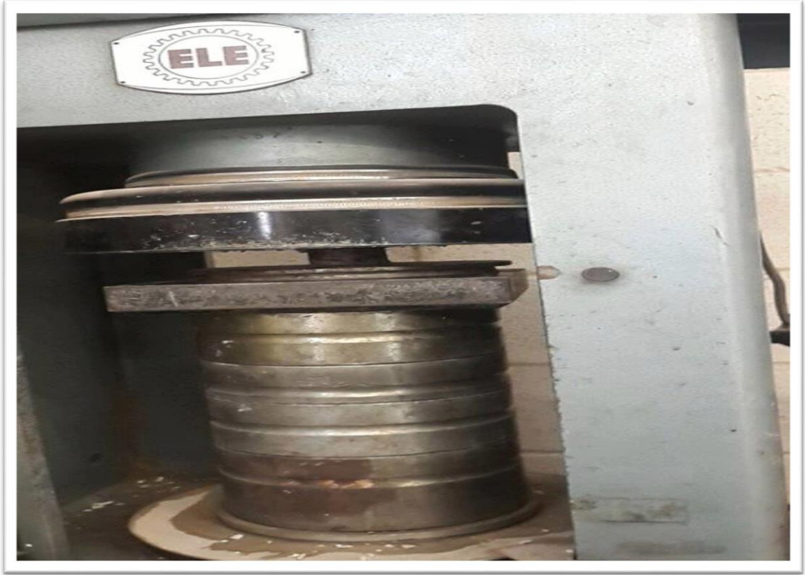
Figure 3.5: An epoxy with EPO sample after 24 hours' compression strength by compression machine.
