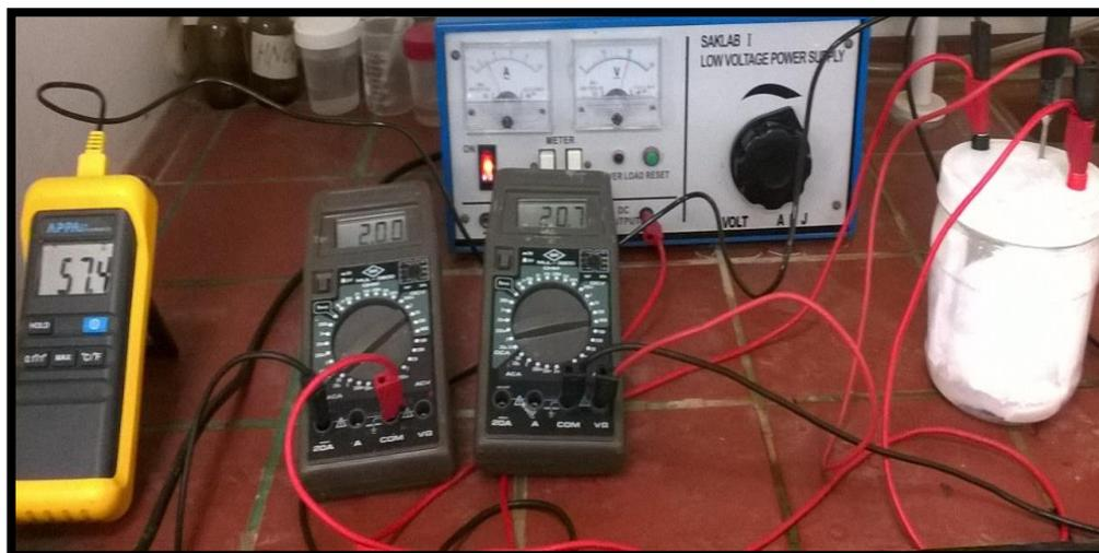
**Fig.(3.8):** Calorimeter set up
