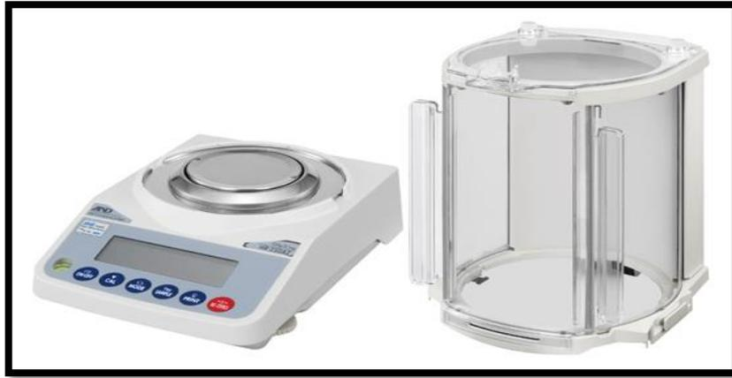
**Fig.(3.5):** The Analytical Balance HR-200
