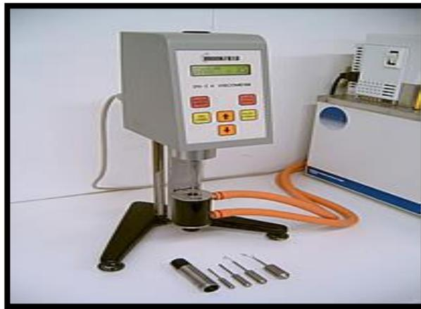
**Fig.(3.2):** Brookfield Digital Viscometer Model DV-I+
