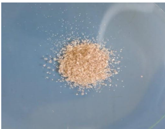
Figure 2.4: Cellulose Modified with 2,6-Pyridine dicarbonyl dichloride Product.
