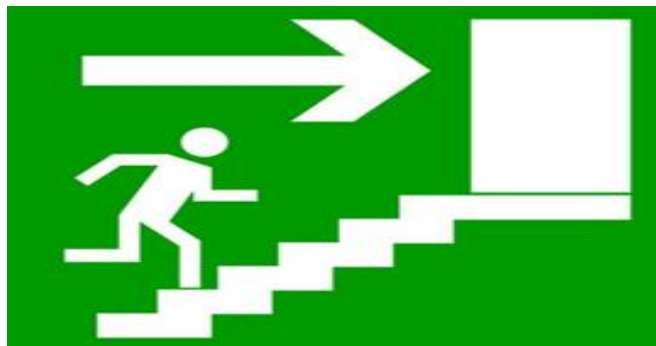
Figure 211 Exit sign for basement floors
