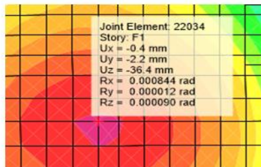
Figure 86 LTD deflection in selected panel
