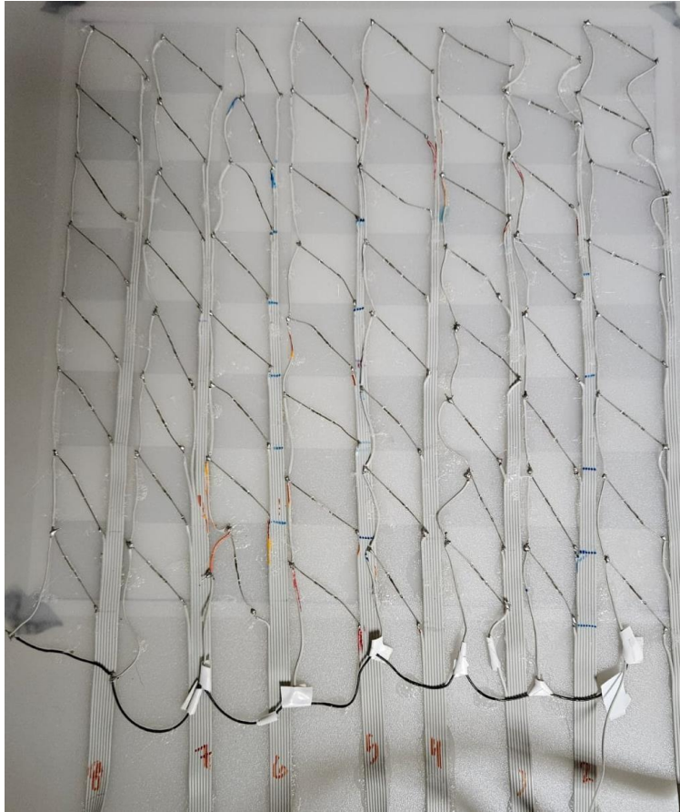
Figure 6 64 Reed Switches wiring
