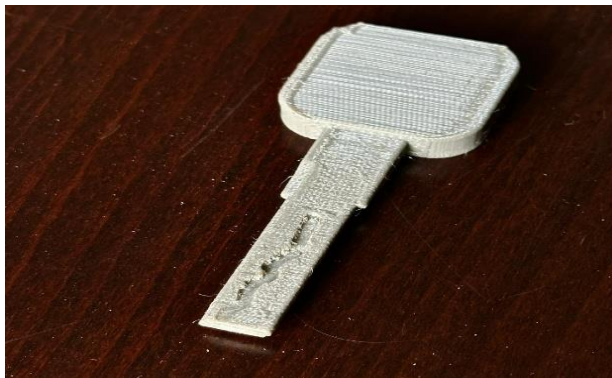
Figure 17: 3D-printed PLA prototype key used for toolpath and groove geometry validation
