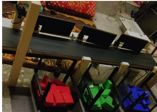
Figure 3.2: Conveyor Belt That Objects Placed On to Be Sorted
