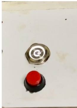
Figure 3.1: Power Button and Push Button to Turn the System ON and OFF
