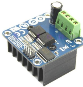
Figure 3.5: BTS7960 High Current 43A H-Bridge Motor Driver
