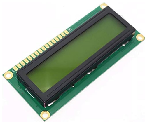
Figure 4.11: 16x2 LCD Screen
