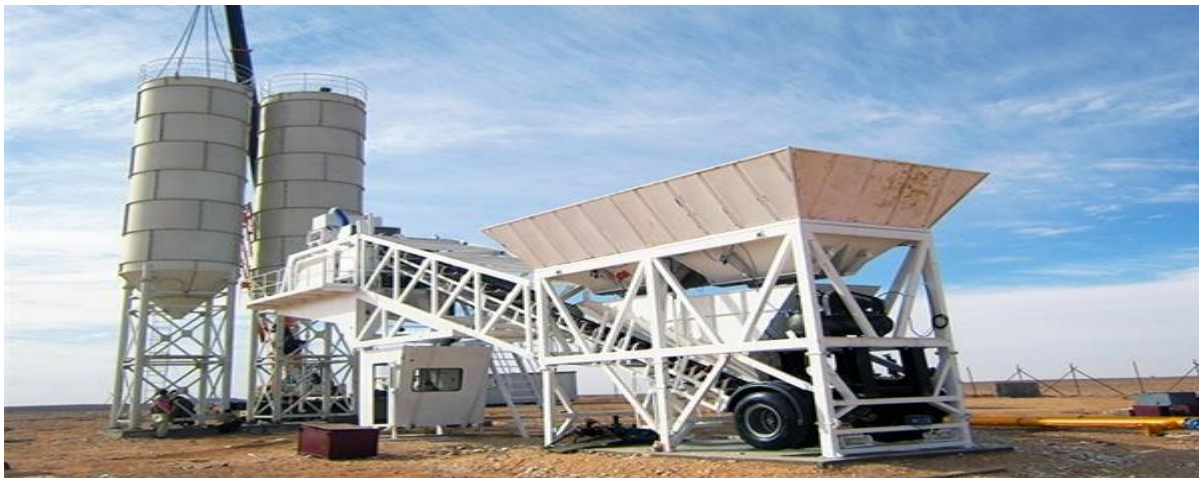
Figure 5: Mobile concrete plant
