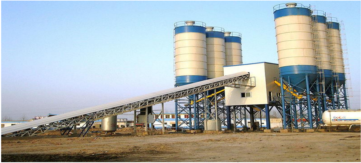
Figure 6: Stationary concrete plant
