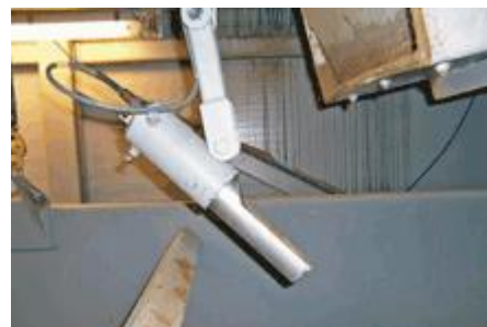
Figure 13:Moisture Sensor located under Aggregate Bin
