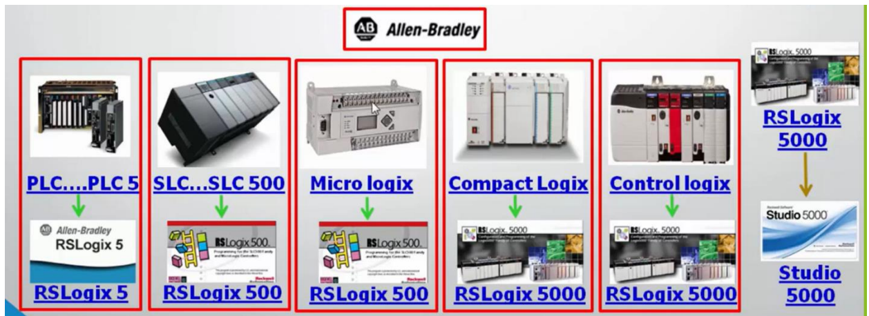
Figure 34:Allen-Bradley PLC and Program
