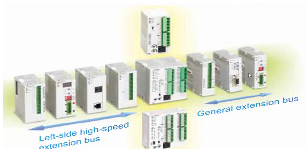
Figure 58 :Connecting Extension Modules to Delta PLCs
