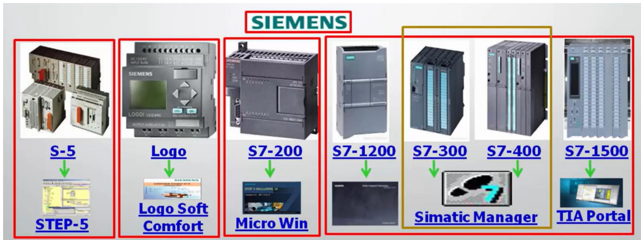
Figure 31: Siemens PLC and Program
