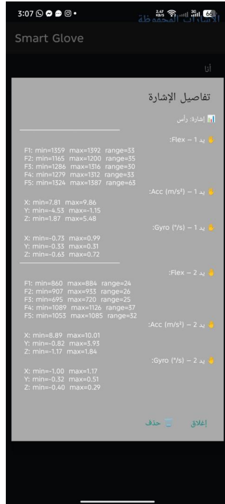
Figure 4: Data for the word "رأس" that was recorded and contains 22 values, which are 5 values for flex sensors and 6 values for MPU (Accelerometer, gyroscope) for each hand.
