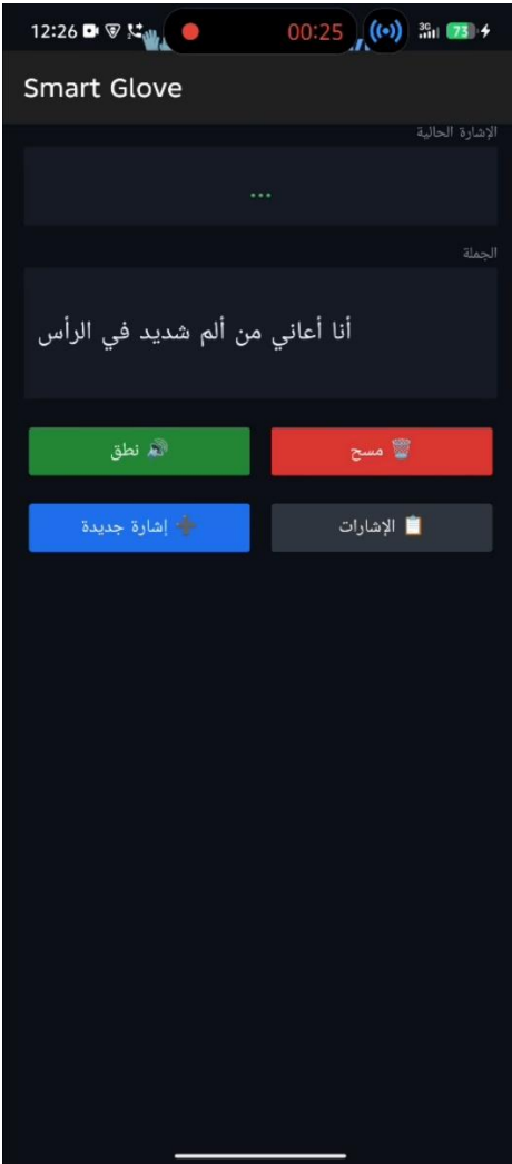
Figure 3: After performing the movements of 3 words, which are "ألم", "رأس", "أنا", the AI intervenes and rearranges the sentence to become "أنا أعاني من ألم شديد في الرأس"
