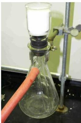
**Figure 1.5:** Dry column flash chromatography setup
