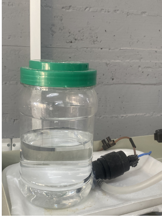
Figure 4.3: Water Tank and Pump
