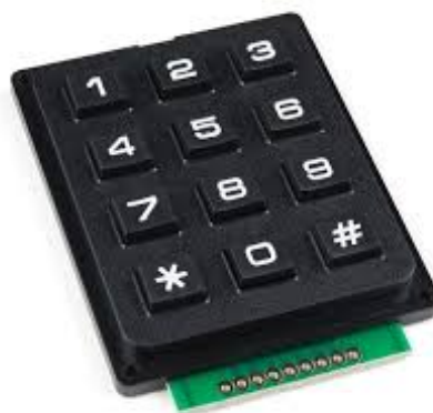
Figure 3.11: Keypad interface used for password entry and session configuration
