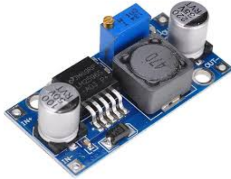
Figure 3.18: LM2596 buck converter module used for voltage regulation
