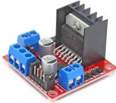
Figure 3.8: L298N Motor Driver Module used to control DC motors
