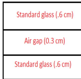
Figure 9.10: components of windows after insulation. [5]
