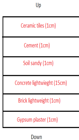
Figure 9.7: Components of roof before insulation. [5]
