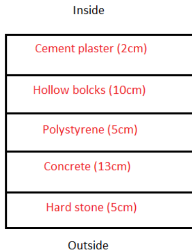
Figure 9.8: Components of external walls after insulation. [5]
