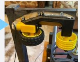
Motor Mount: to cap the bottle
