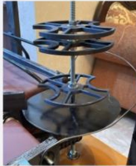
Star Wheel: to carry the bottle during capping process
