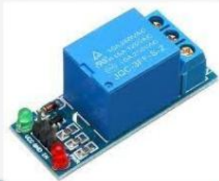
Two Relay Modules: to switch electrical devices or systems on and off
