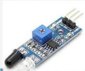
Two IR sensors: the 1st to detect the bottle to start filling and the other one to detect bottle for capping
