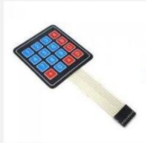
Keypad: press "#" to start the project
