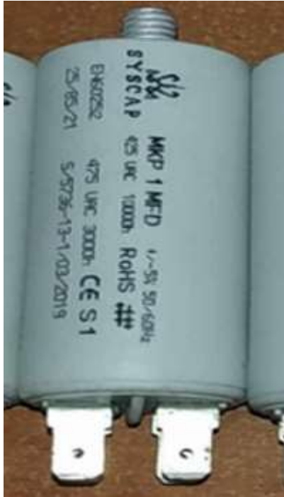
Figure 26 :We used a test capacitor with a value of 1 \mu\text{F} .
