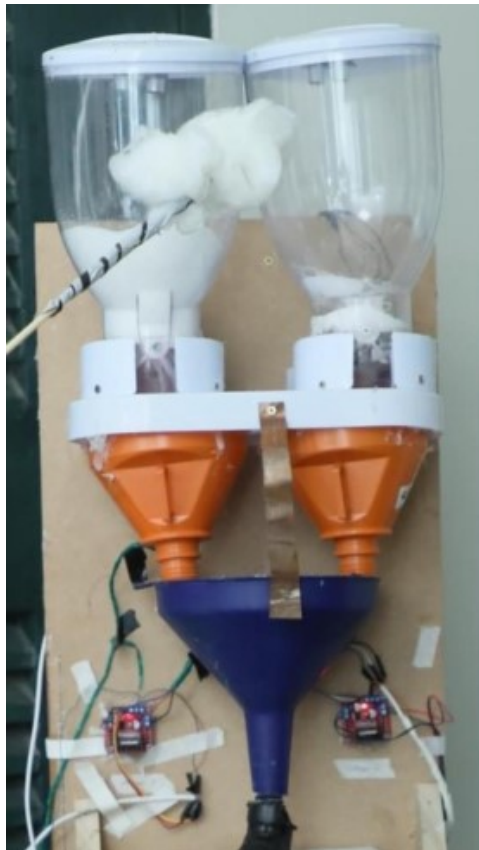
Figure 21: Sugar Dispensing structure.
