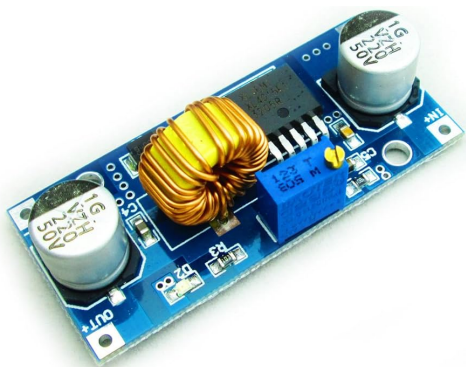
Figure 7: XL4015 Voltage Regulator
