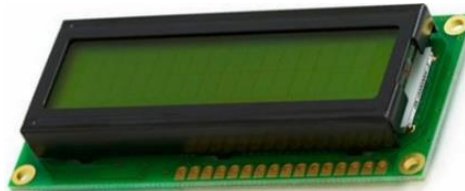
Figure 12: LCD Display (16x2)
