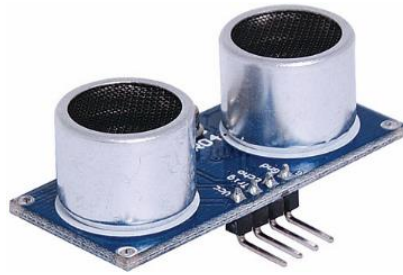
Figure 9: Ultrasonic Sensors (HC-SR04)
