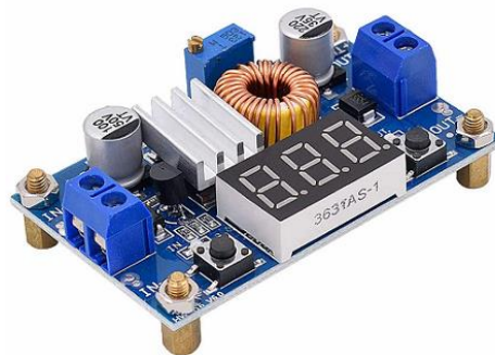
Figure 10: XL4015 Adjustable DC-DC Buck Converter With 3-Digit 7-Segments display
