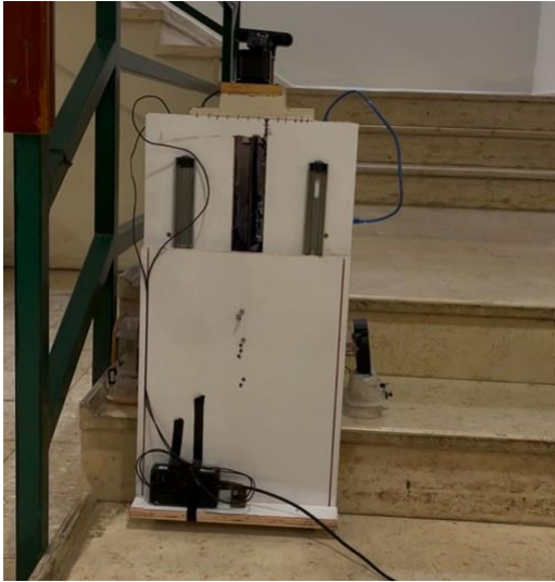
Figure 3.9: Robot Moving Left Across the Step During Cleaning
