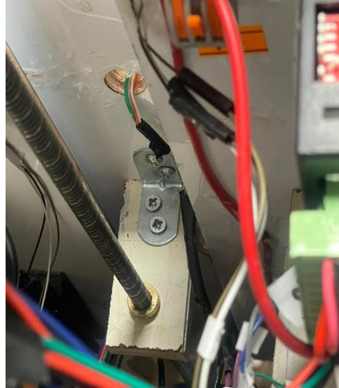
Figure 3.13: Angle Bracket Connection for Lead Screw.
