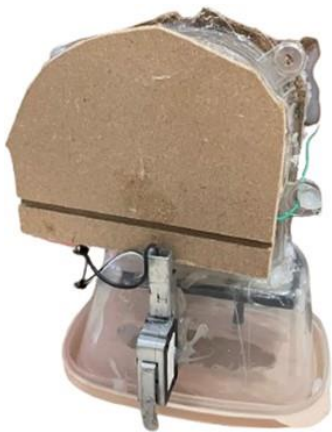
Figure 3.19: Dust Collector Fan One.
