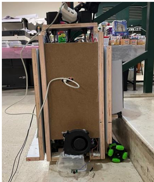
Figure 3.11: Back Cuboid Raised After Step Cleaning Completion.
