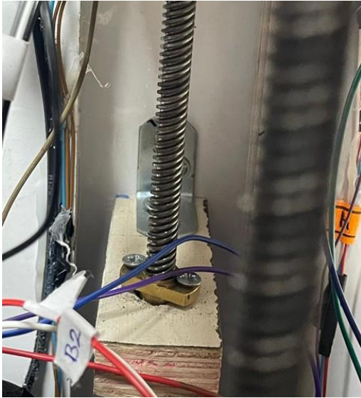
Figure 3.12: Close-up of Lead Screw and Nut Mechanism.
