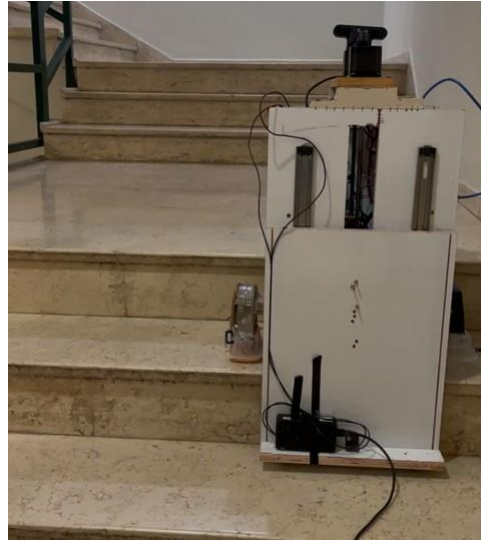
Figure 3.10: Robot Moving Right Across the Step During Cleaning
