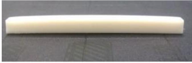
Figure 16: Warping of 3D printed part due to stress build-up
