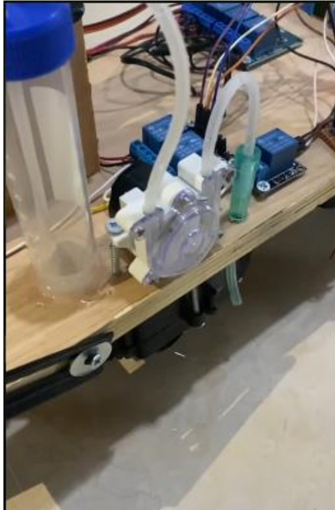
Figure 17: Water pumps on agricultural robot
