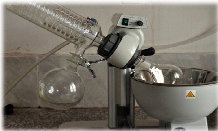
Figure (2.1) Rotary evaporator used for drying plant extracts under reduced pressure.
