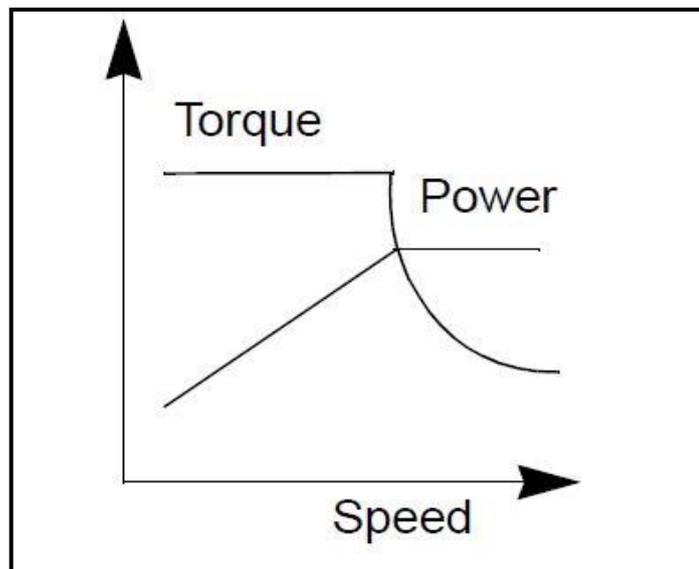
**Figure (5.7) :** Constant Power & Constant Torque Loads [28].
