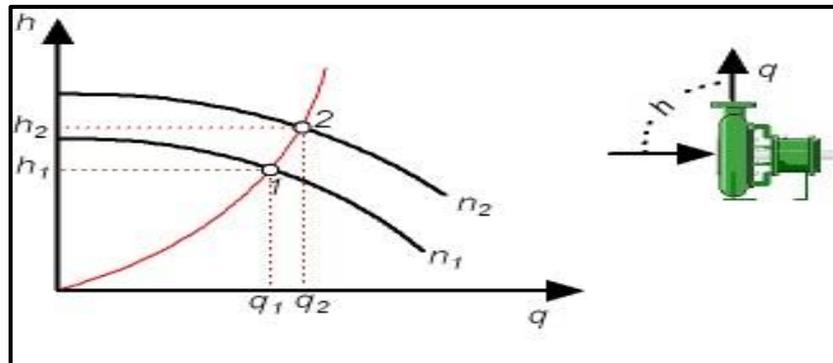
**Figure (3.7):** change in pump characteristic through changing the wheel velocity.
