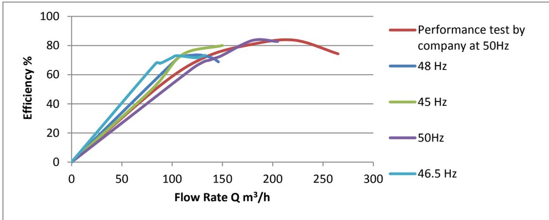
**Figure (6.13):**flow rate versus Efficiency of pump at deferent speeds.
