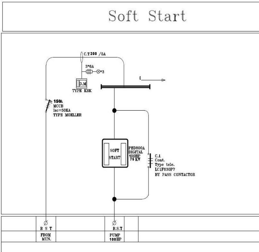
**Figure A2:** Power Circuit of the Control System
