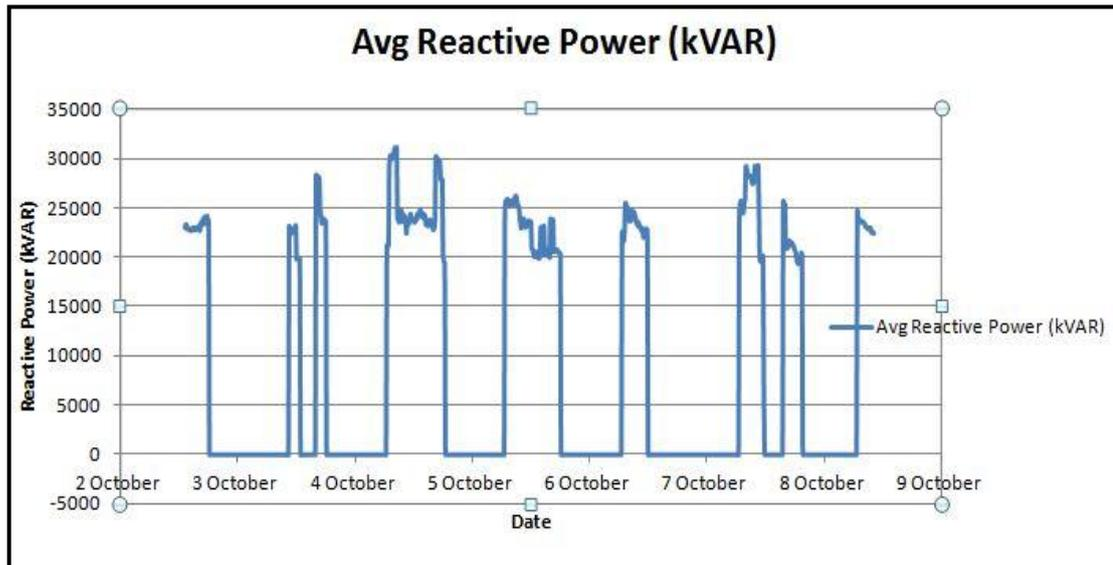
**Figure (6.11):** Average reactive power for irrigation company pump
