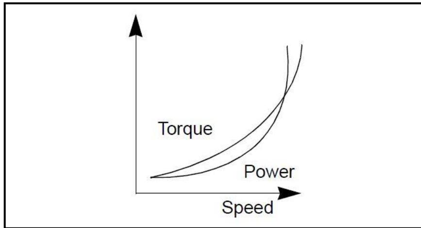
**Figure (5.5)** :Variable Torque, Variable Speed Loads [28].
