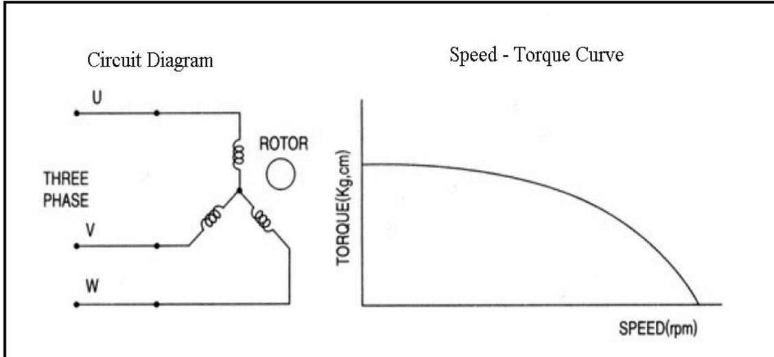
**Figure (5.1) :** Speed – Torque curve for induction motor [27].
