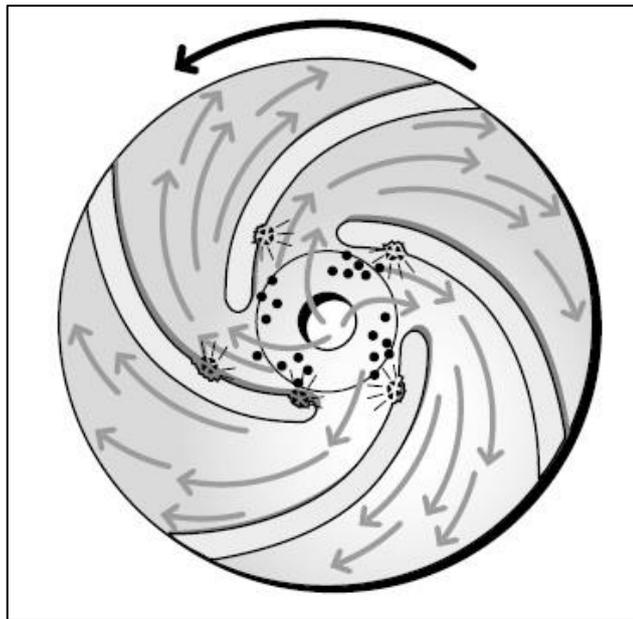
**Figure (3.2.3):** Cavitations on impeller.
