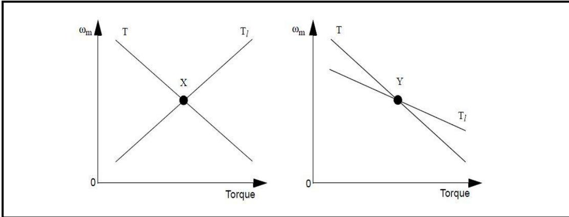
Figure (5.3) :Torque-Speed Curve – Same Motor with two different loads [28].
