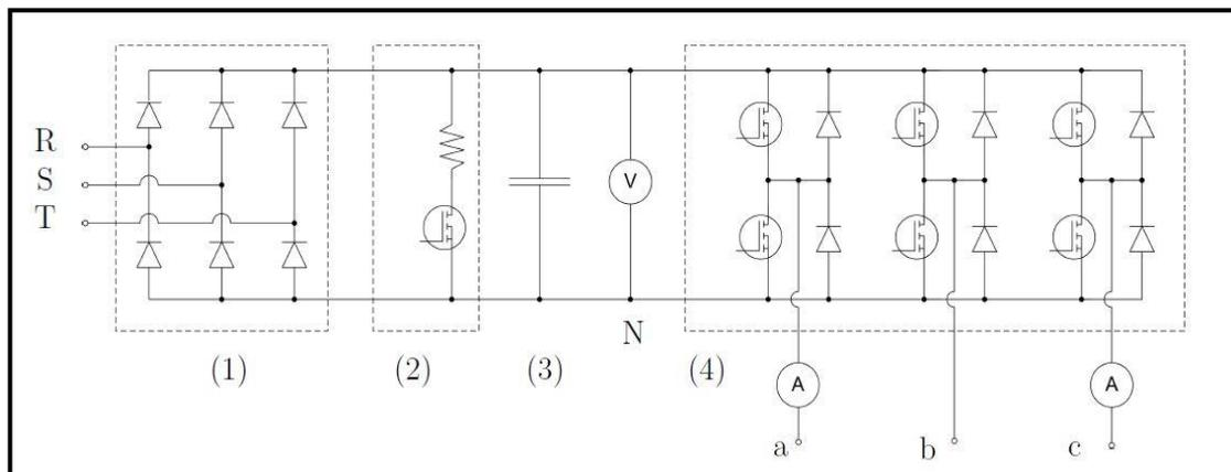
**Figure (5.10)** :A typical frequency converter.
