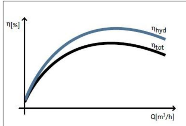
**Figure (3.2.3):** Efficiency curves for the pump ( $\eta_{hyd}$ ) and complete pump unit with motor and controller ( $\eta_{tot}$ ).
