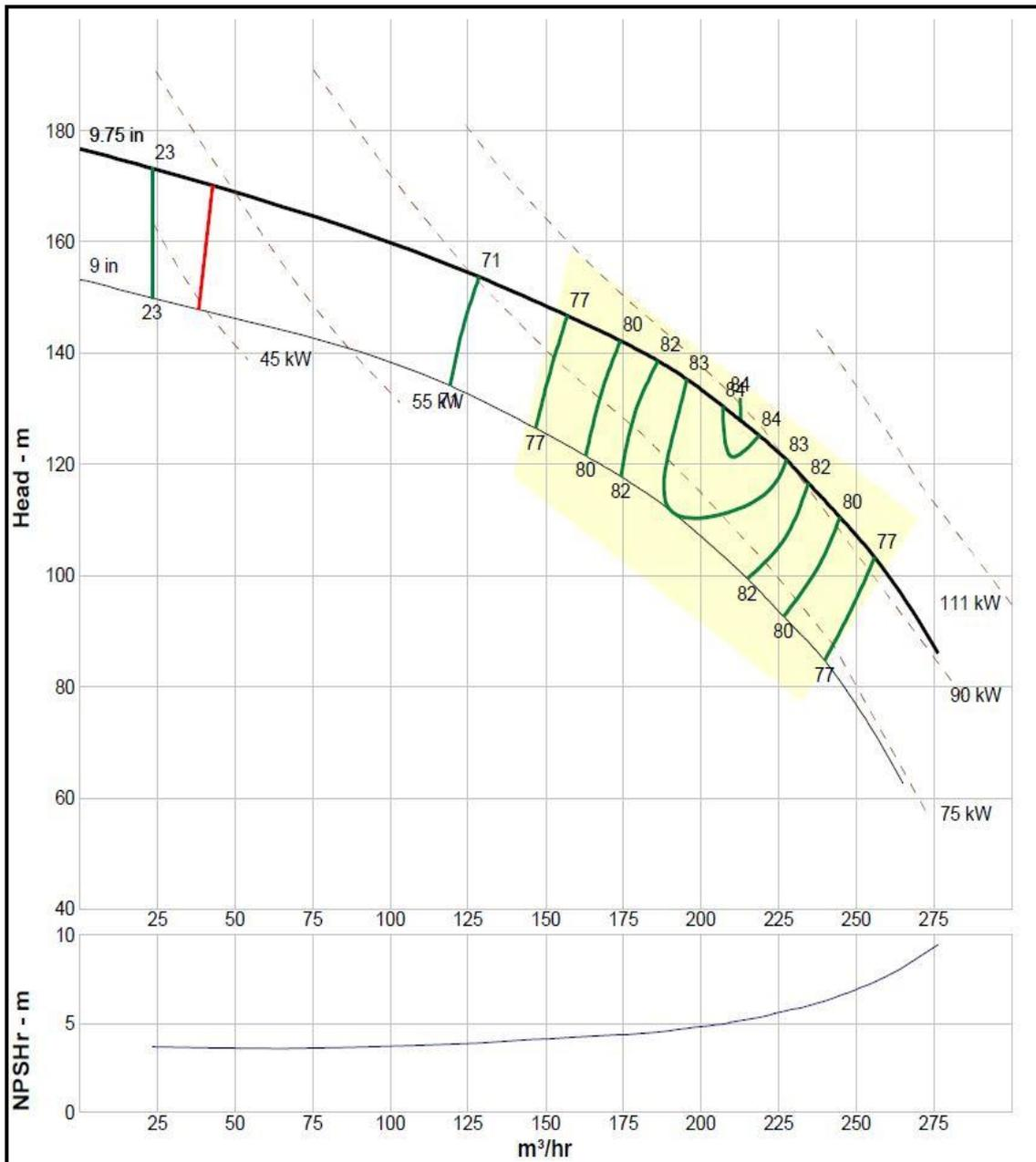
**Figure (4.2) :** Design curve of Agricultural Irrigation Company pump [21].
