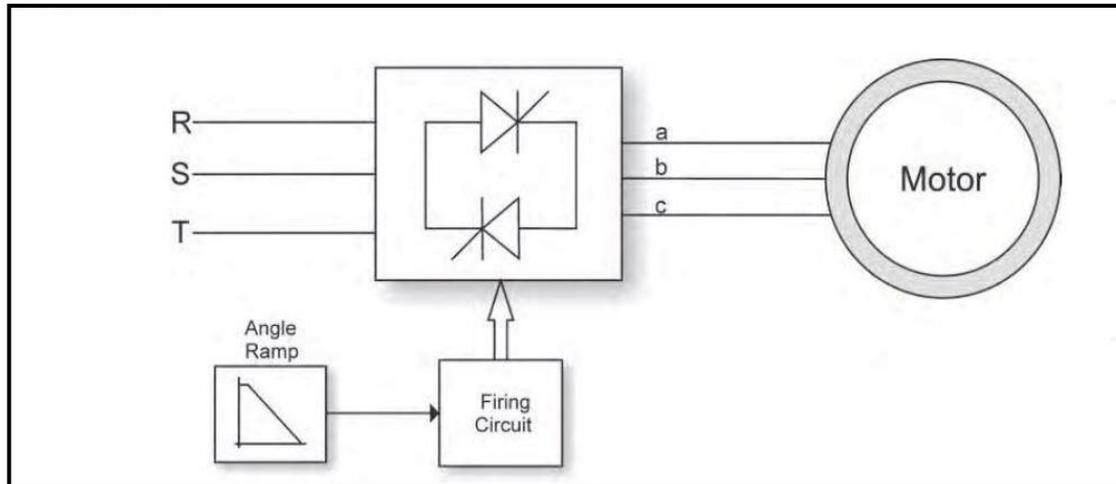
**Figure (5.9)** :Basic block diagram of the voltage-ramp technique[30].
