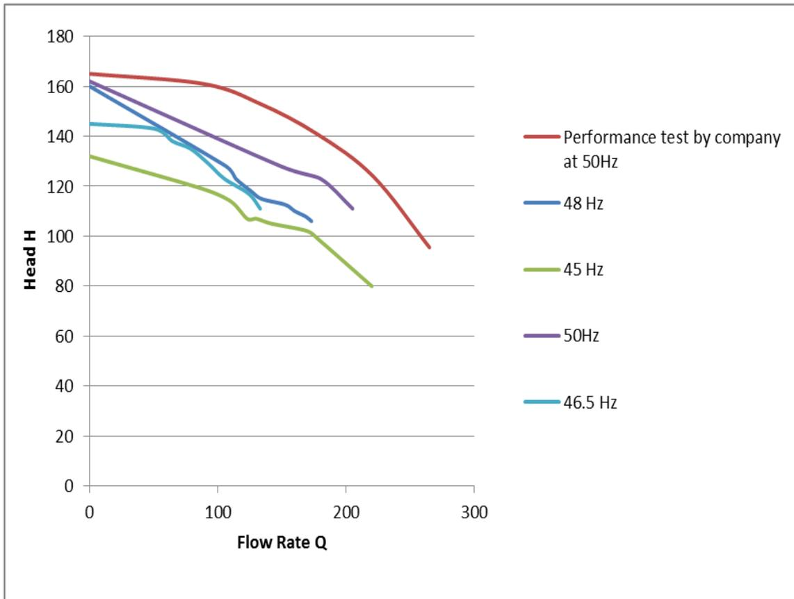
**Figure (6.12) : Effect of speed variation on pump characteristics**
