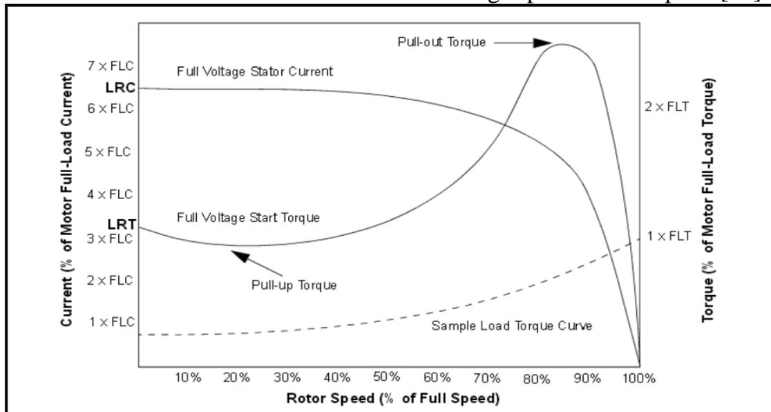
**Figure (5.2) :** Typical Torque-Speed curve of 3-PHASE AC Induction motor [28].
