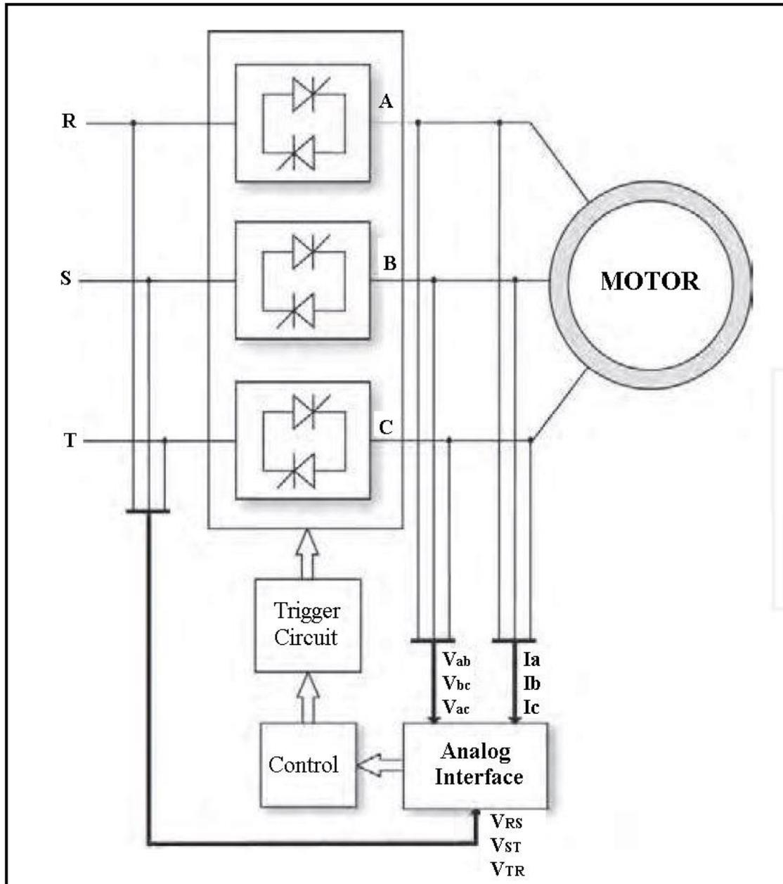
**Figure (5.8)** :Basic diagram of soft starter[30]
