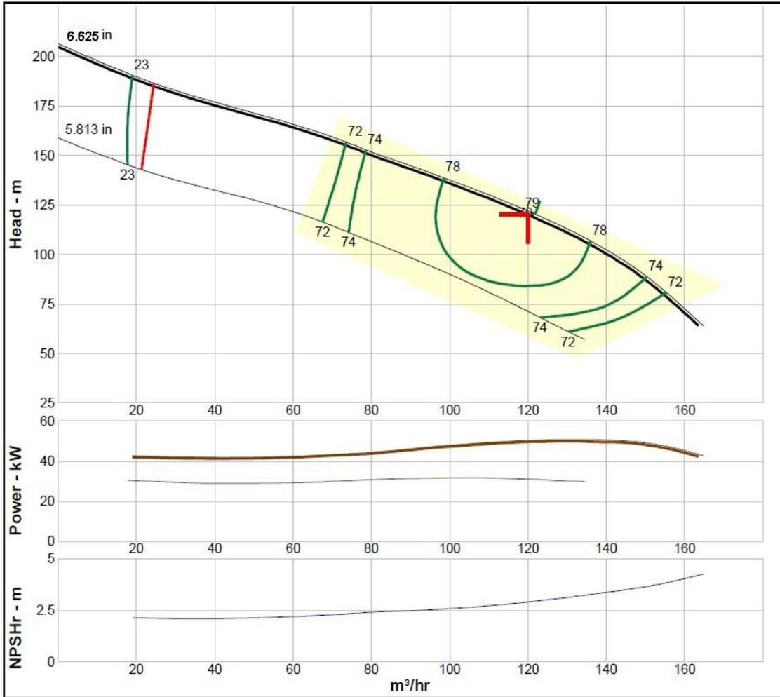
**Figure (4.3) :** Design Curve of Waleed Ribhi well pump [21].
