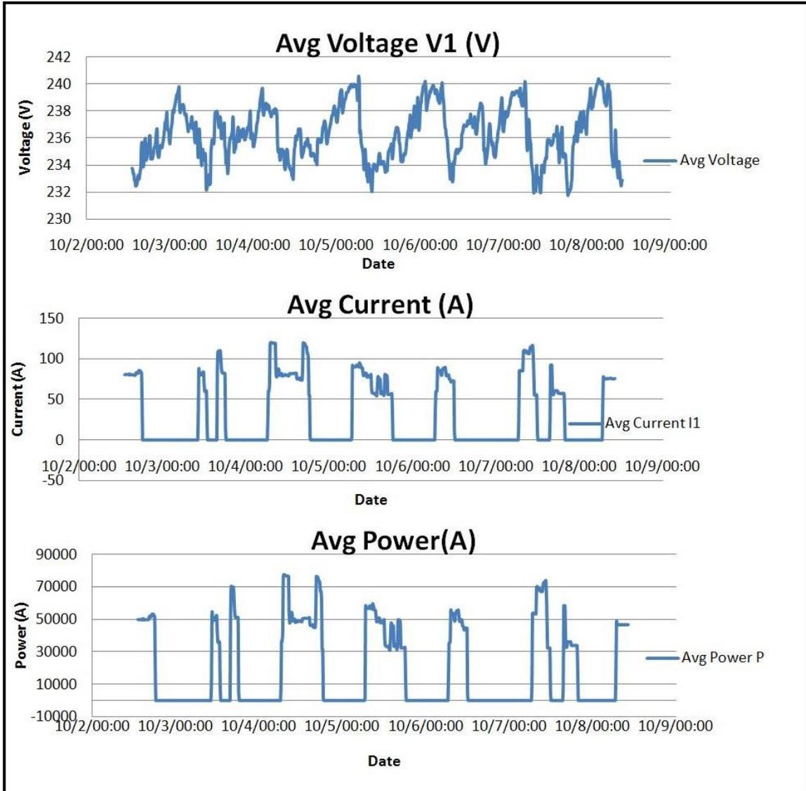
**Figure (6.9):** Average voltage ,current ,total power for Abu saleh pump during second testing period
