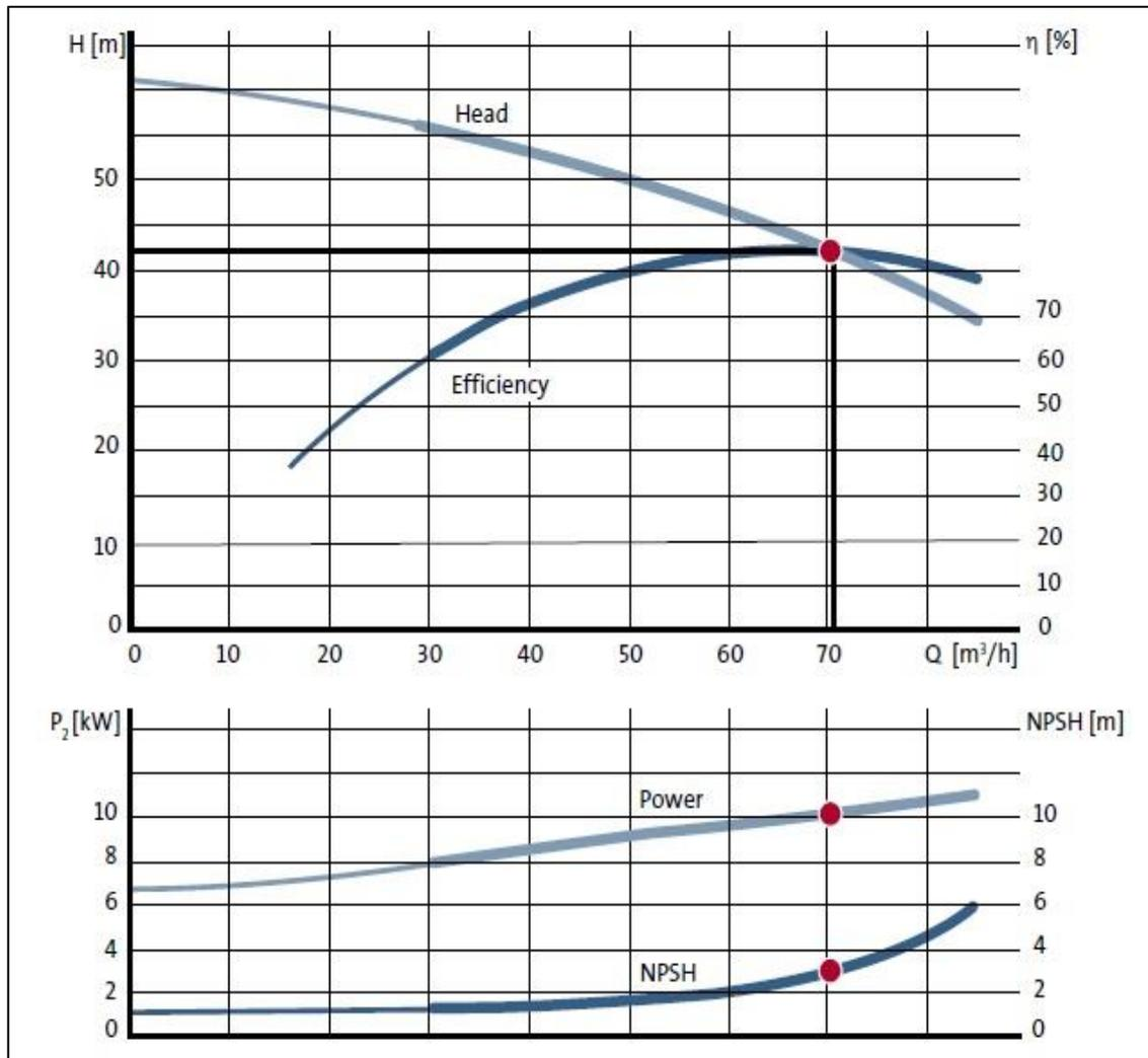
**Figure(3.3):** Typical performance curves for a centrifugal pump [5].
