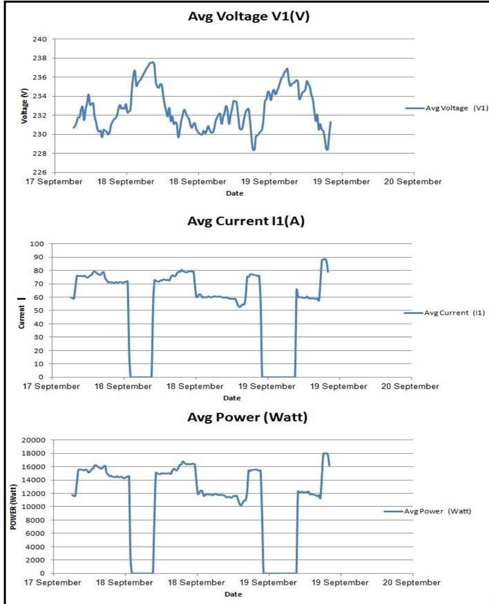
**Figure (6.14)** :Average voltage ,current ,total power for Waleed Ribhi pump during second testing period
