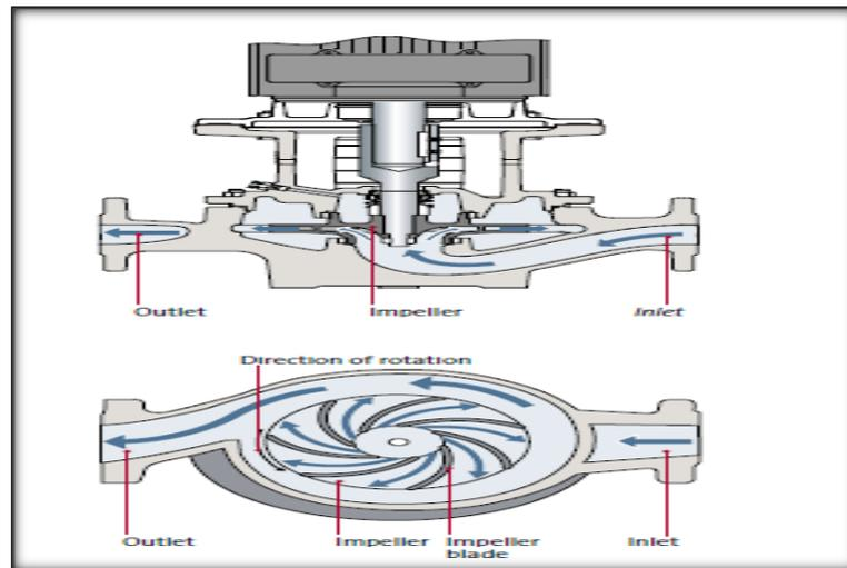
**Figure(3.2):** Hydraulic components of centrifugal pump [5].
