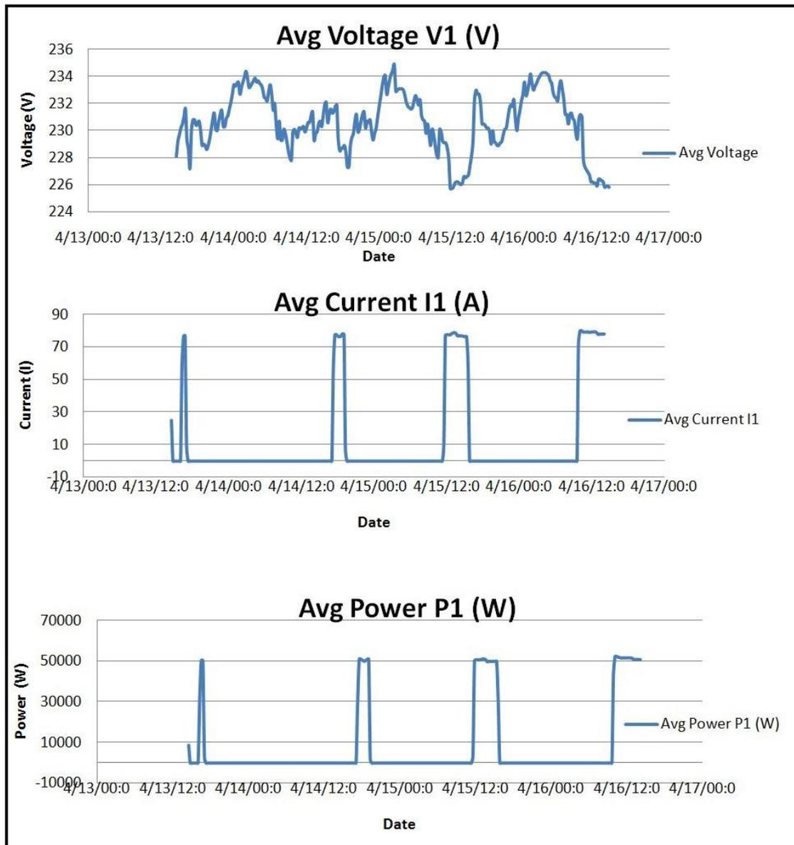
**Figure (6.7):** Average voltage ,current ,total power for Abu saleh pump during second testing period
