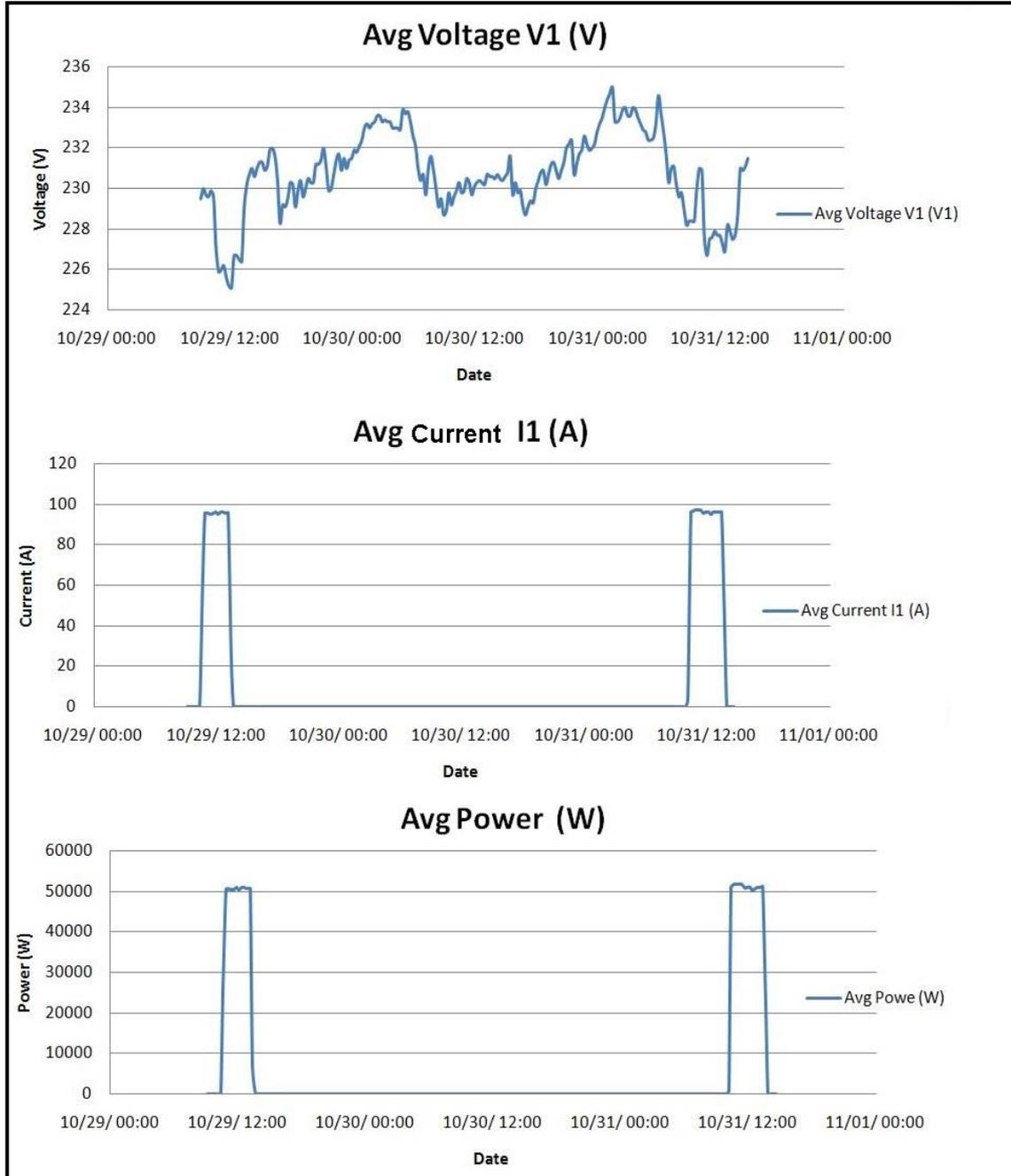
**Figure (6.5):** Average voltage ,current ,total power for Abu saleh pump during first testing period
