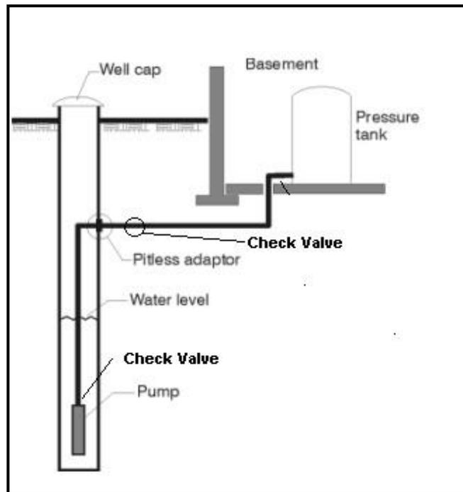
**Figure (6.1) :** Water Pumping System Component
