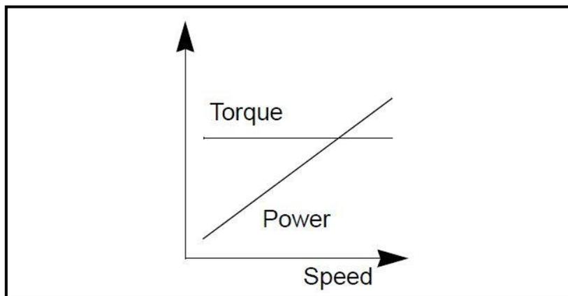
Figure (5.4) :Constant Torque, Variable Speed Loads [28].
