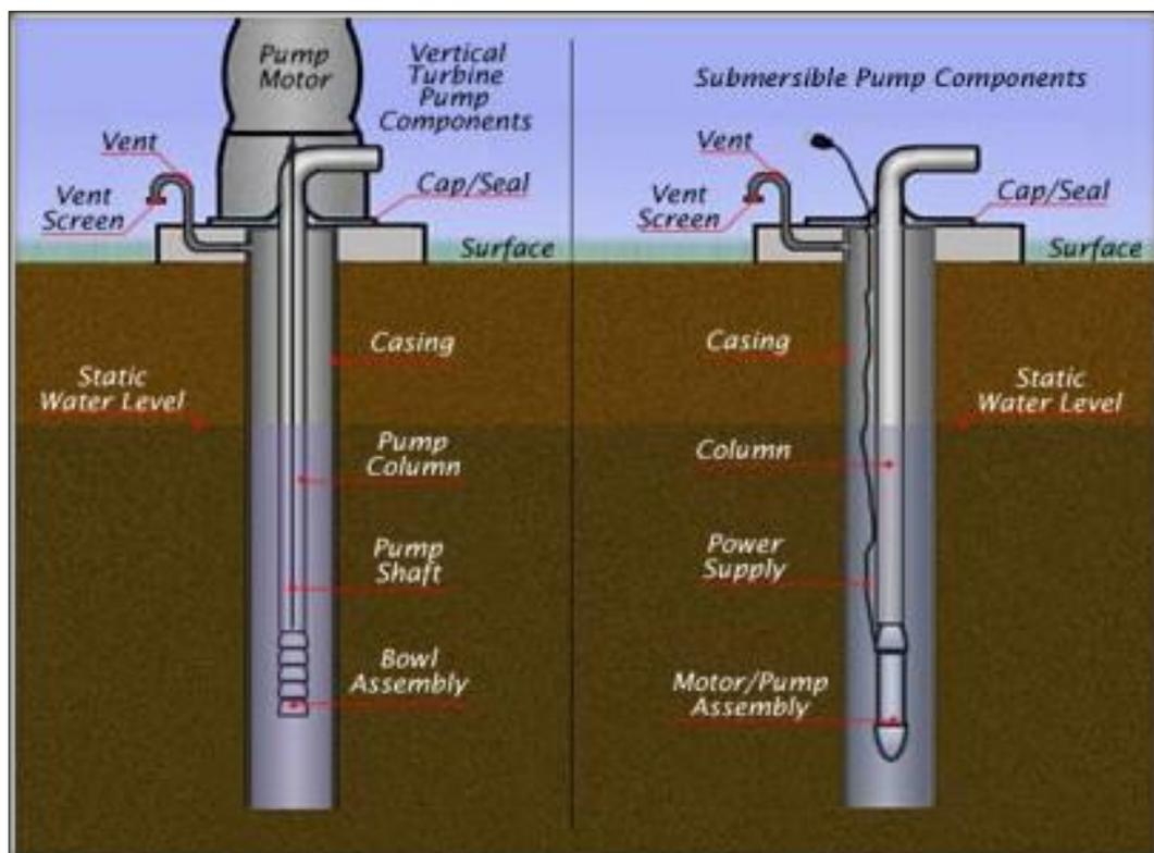
**Figure(3.1):** Type of pumps used in ground water well.
