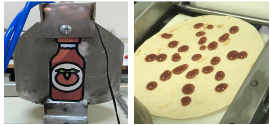
Figure 4: Innovative "Shower" Mechanism for Controlled Ketchup
