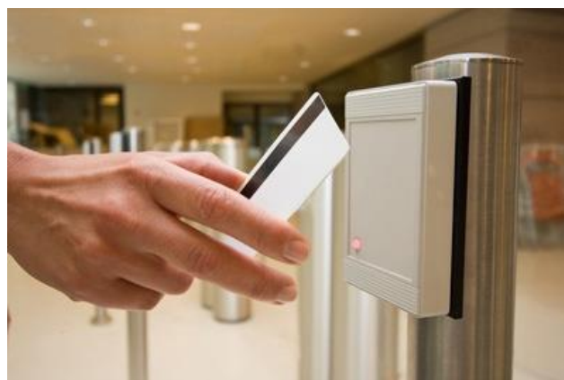
Figure3.15 (Proximity access control )(agtelecom)
