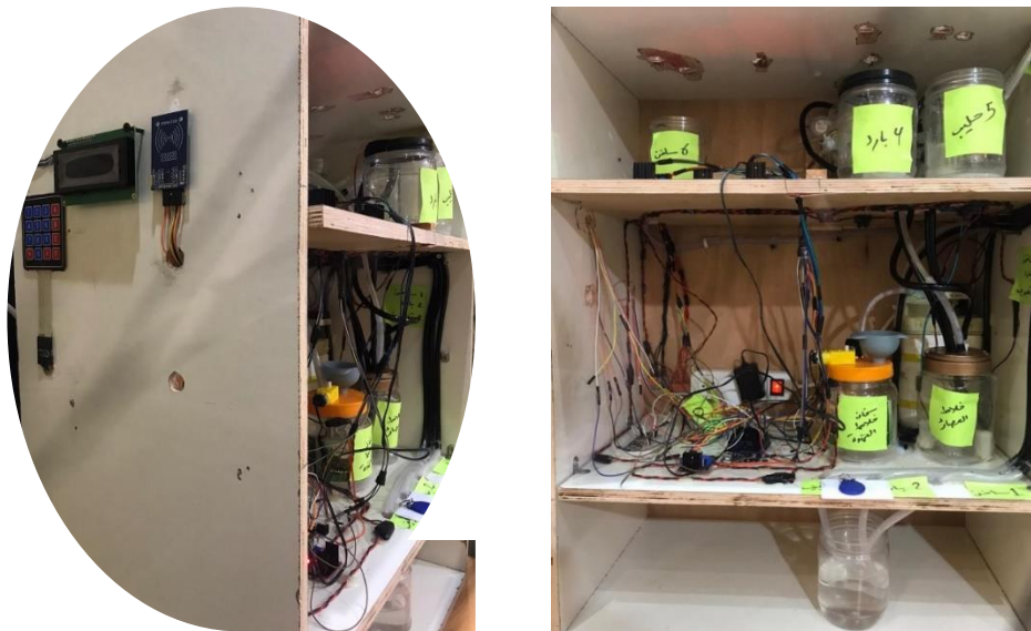
Figure 2: Complete Hardware Layout of iDrink Station Prototype
