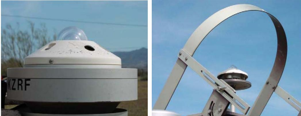
**Figure (3. 3): Pyranometers used for measuring the global radiation (left) and diffuse radiation (right)**
