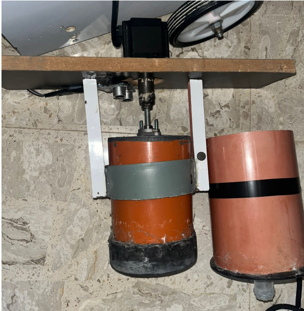
Figure 3.2: Container for pressing and pushing the grout
