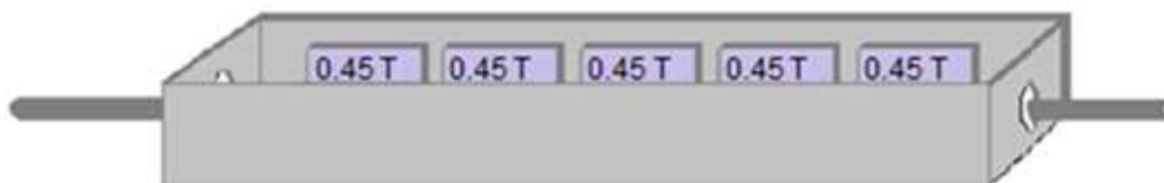
Figure 3.3: scheme of the regular magnetic device used to study the efficiency of the magnetic treatment in different pH values
