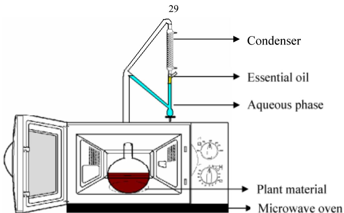
Figure (7): Microwave - ultrasonic apparatus [71]
