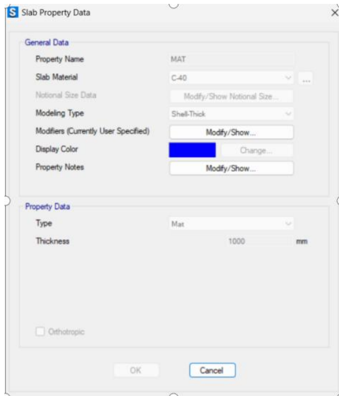
Figure4.97 :footing definition in SAFE.
