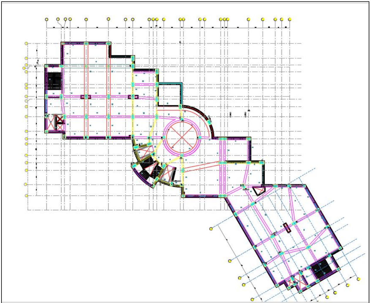
Figure 2.4 Beams distribution (second floor).
