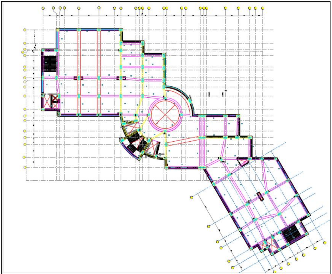
Figure 2.3 Beams distribution (first floor).
