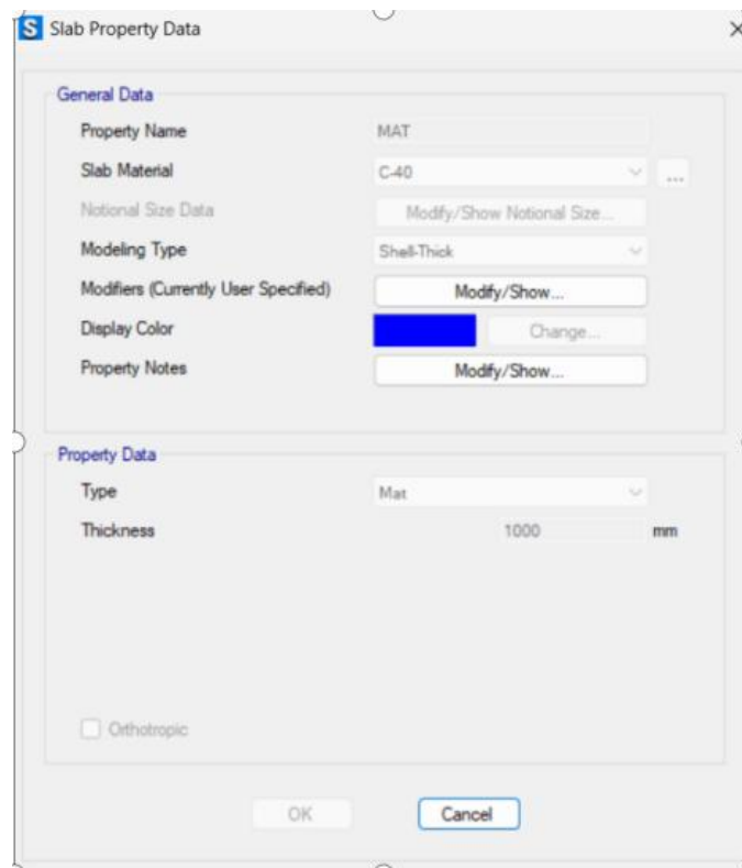
Figure3. 116 :footing definition in SAFE.
