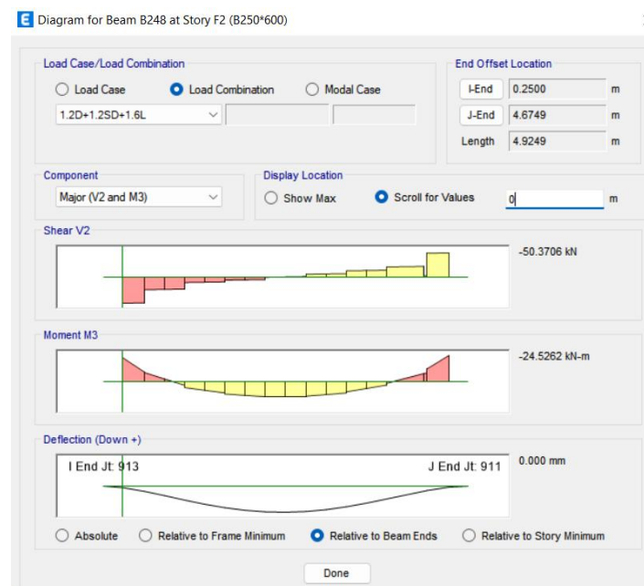
Figure3. 74 moments for beam in the X direction.
