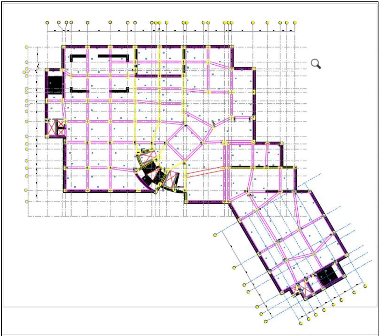
Figure 2.1 Beams distribution (basement one and basement two).
