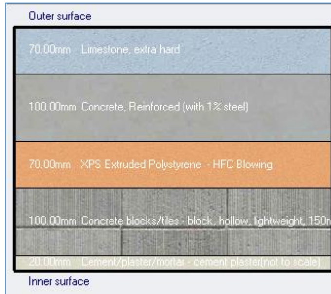
Figure 57 cross-section of the external wall
