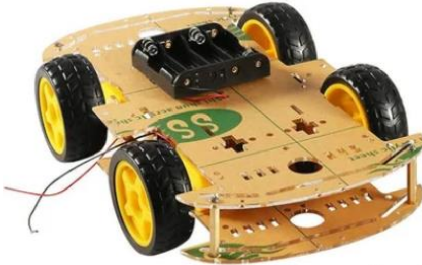
Figure 29: Car Chassis with DC Motors
