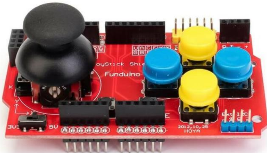
Figure 25: Joystick Shield for Arduino V1.a
