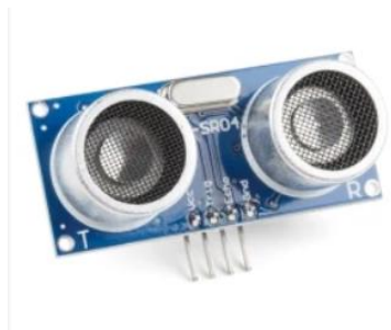
Figure 30: Ultrasonic Sensor (HC-SR04)
