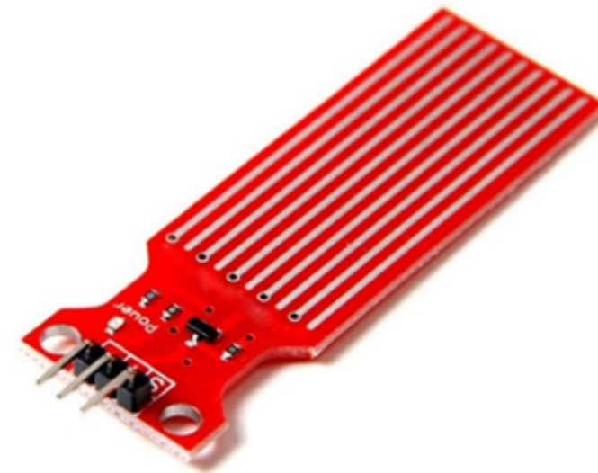
Water Level Sensor
