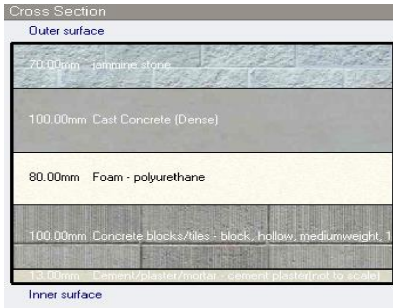
Figure 101 Cross section for external walls.
