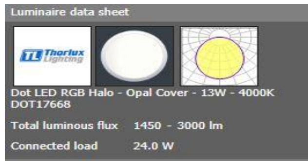
Figure 155 luminaire types chosen to W.C
