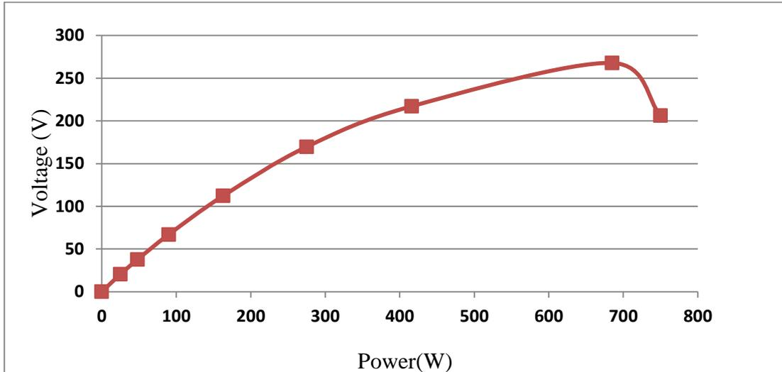
**Figure (4.11):** The relationship between the output power of PEMFC and voltage through variation of the load.
