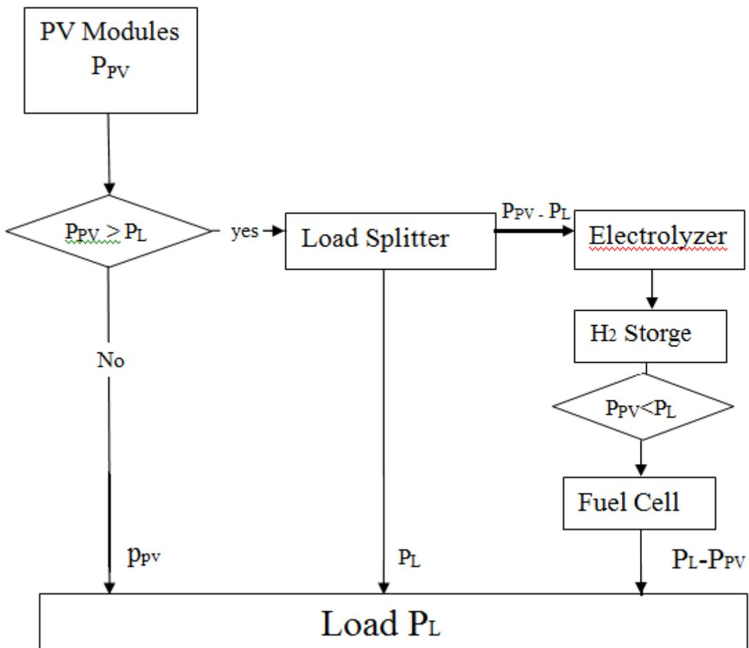
**Figure (5.3):** Logical block diagram for PMS.
