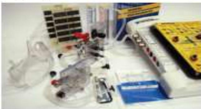
*The Emona HELEx Add-in Module along with kit components including Photovoltaic Cells, Hydrogen Fuel Cells and Electrolyzer, which when patched together to implement 17 sustainable energy experiments.*
