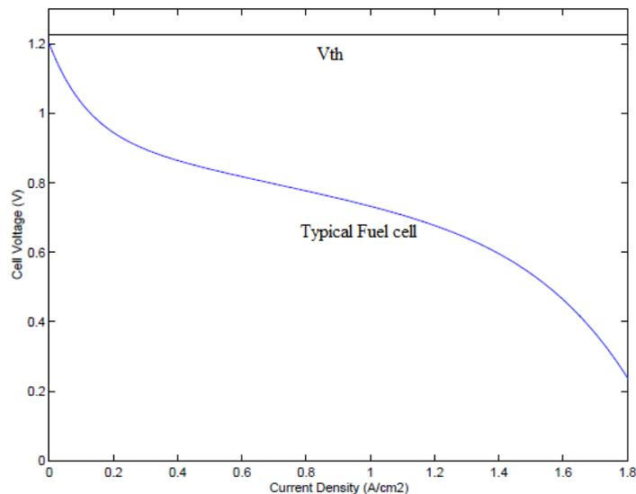
**Figure (3.6):** The V-I characteristic of PEM fuel cell.
