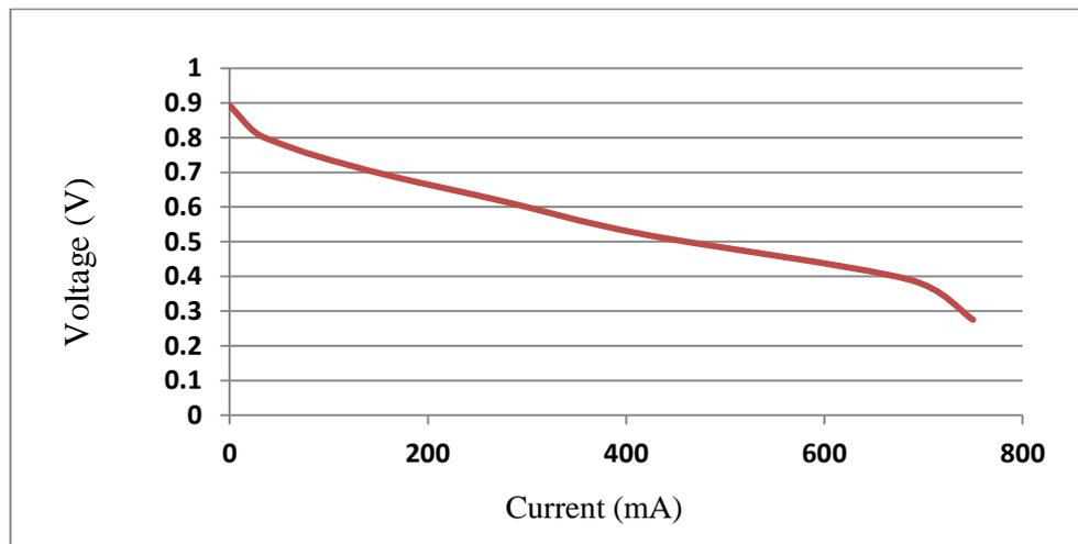
**Figure (4.10):** The (V-I) characteristics of PEMFC.
