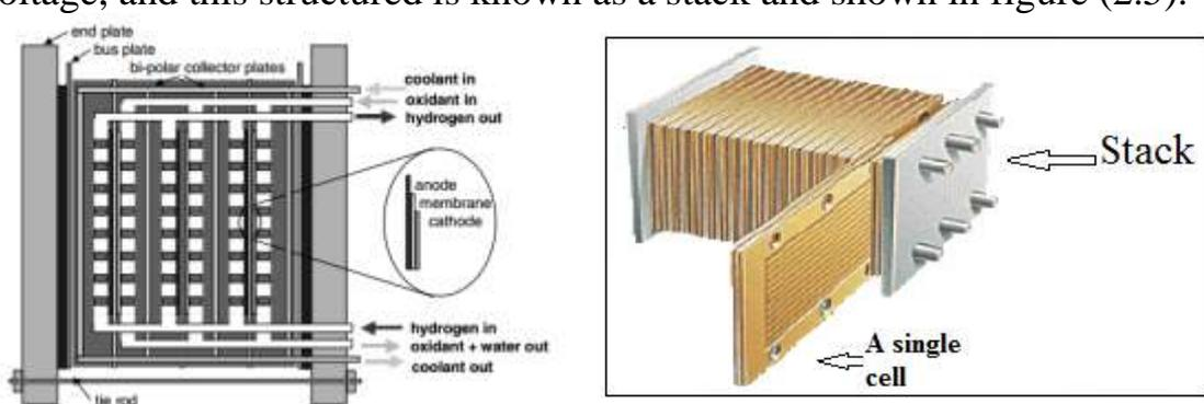
**Figure (2.9):** A collection of fuel cells (stack) to increase the voltage.
