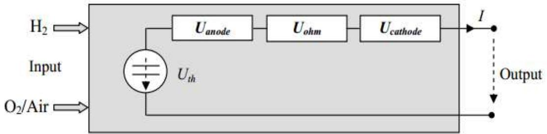
**Figure (3.7):** An equivalent circuit of the actual PEM fuel cell.
