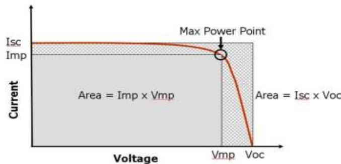
**Figure (2.5):** The I-V curve of a PV module for defining the FF.
