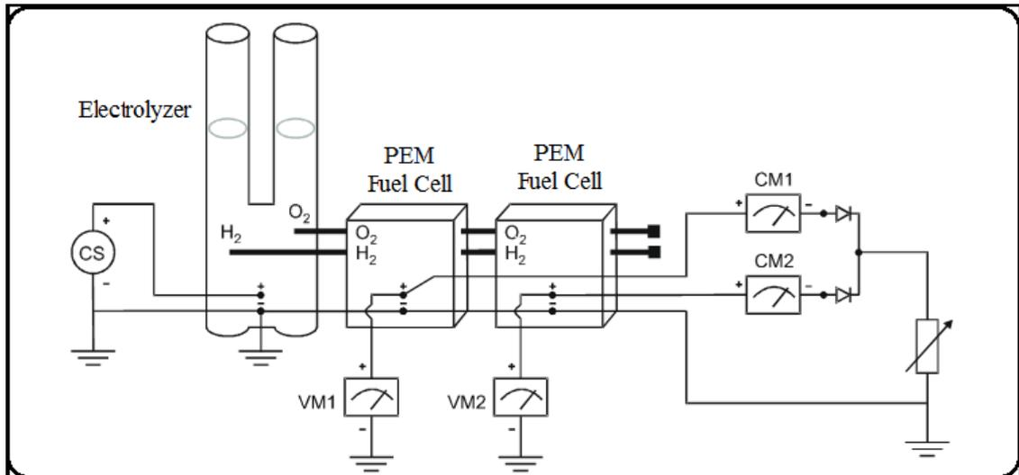
**Figure (4.13):** Two PEM Fuel Cell are connected in parallel.
