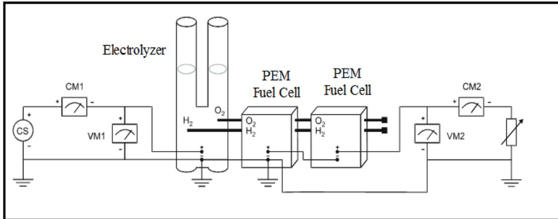
**Figure (4.12):** Two PEM Fuel Cell connected in series.
