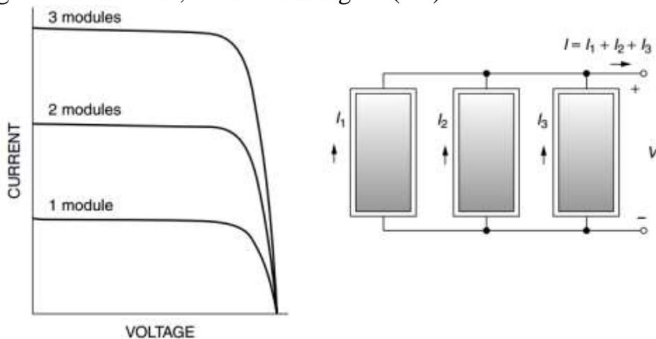
**Figure (3.4):** The I-V characteristics of 3 PV modules connected in parallel.
