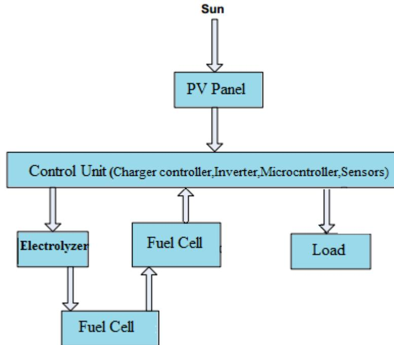
**Figure (2.1):** Block diagram of the Photovoltaic with fuel cell system.
