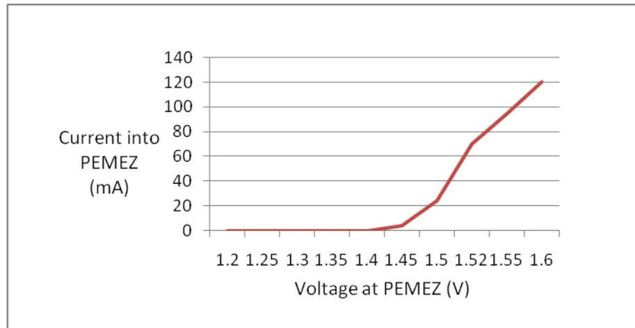
**Figure (4.7):** I-V characteristics of the PEM electrolyzer.
