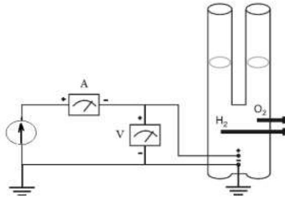
**Figure (4.6):** Current source supplying the electrolyzer .
