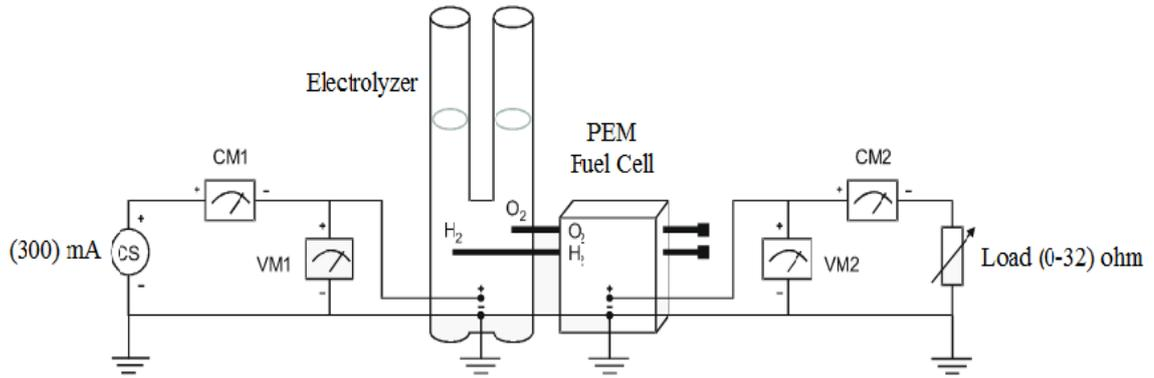
**Figure (4.9):** (PEM) Fuel Cell connection with the electrolyzer , load and measuring devices
