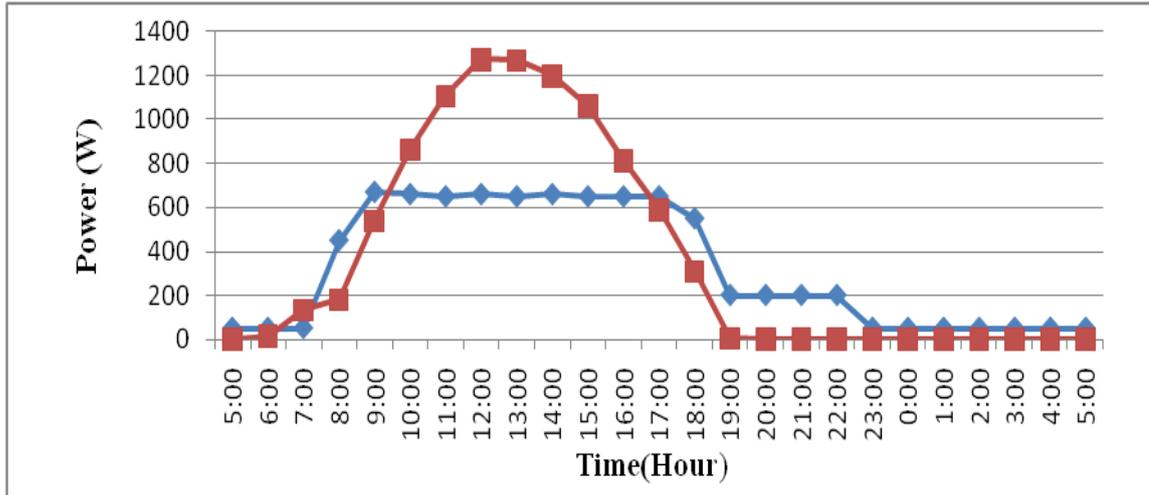
**Figure (5.4):** The load demand and the output power of the PV generator.
