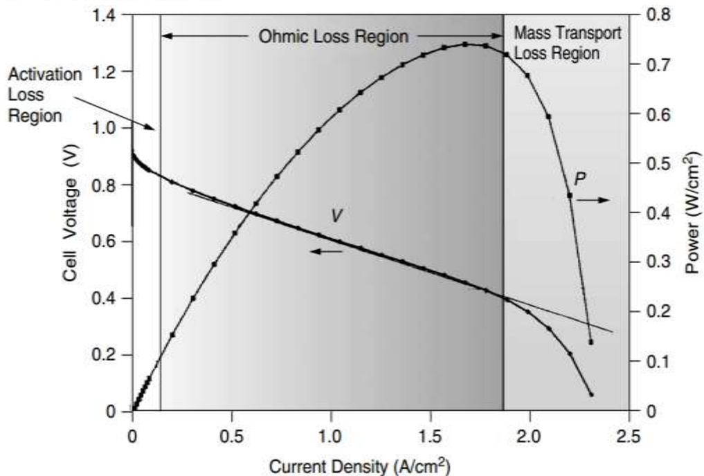
**Figure (3.8) :** The P-V of the PEM fuel cell[10].
