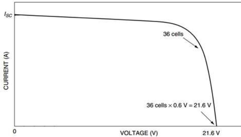
**Figure (3.2):** The I-V characteristics of a typical PV module consisting of 36 cells connected in series. [10].
