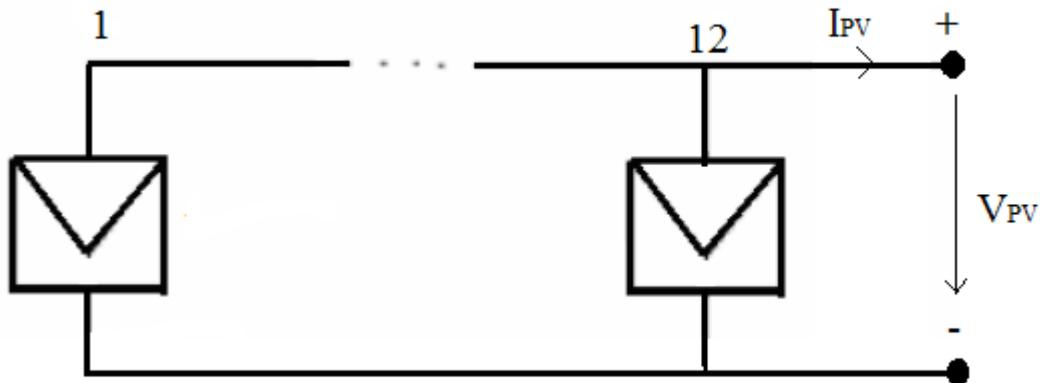
**Figure (5.7):** Connection of the PV modules to build the PV generator
