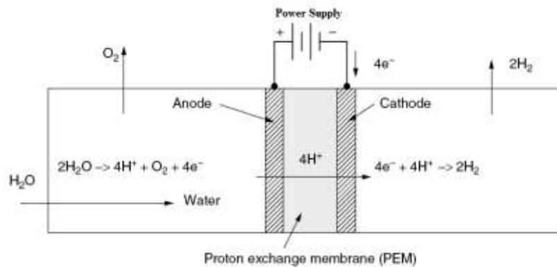
**Figure (2.6):** Principle of PEM electrolyzer.
