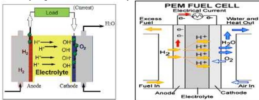
**Figure (2.7):** Basic principle of a PEM Fuel Cell
