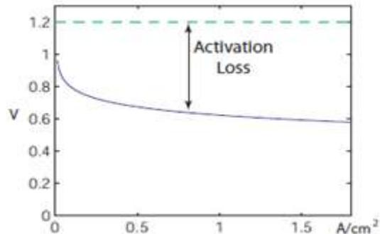
**Figure (3.9):** The V-I characteristics of PEM Fuel Cell affected by the activation losses.
