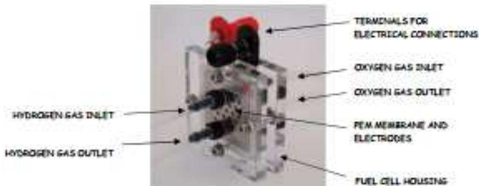
Fig.2 - PARTS OF THE PEM HYDROGEN FUEL CELL
