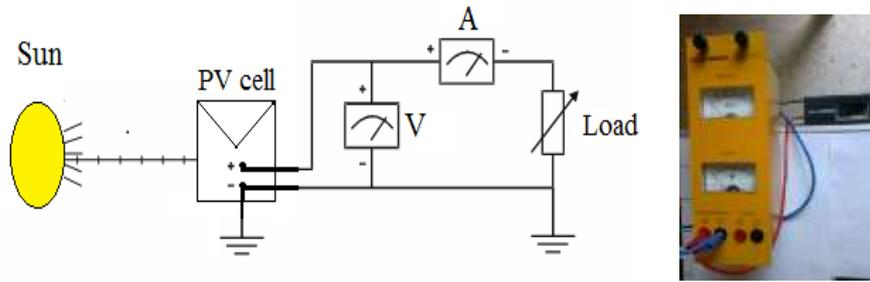
**Figure (4.3):** Measuring circuit for determination of the I-V and P-V characteristics of a PV module.
