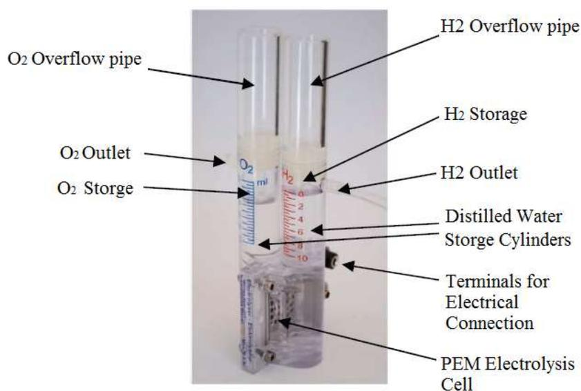
**Figure (4.5):** The PEM electrolyzer used in the experiments to produce H<sub>2</sub> and O<sub>2</sub>.
