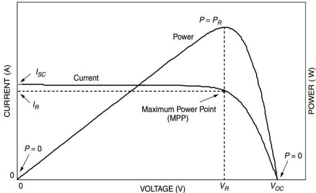
**Figure (2.4):** The I-V and P-V characteristics of typical PV module [10].
