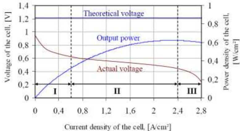
**Figure (2.8):** The V-I and V-P curves of a PEMFC.
