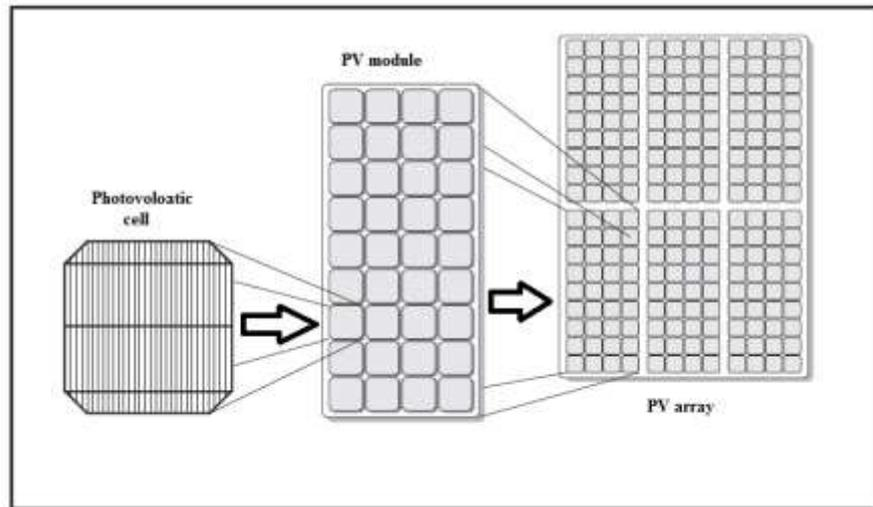
**Figure (2.2):** Photovoltaic cell, PV module and PV array.
