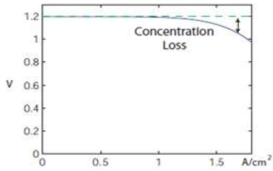
**Figure (3.11):** The V-I characteristics of PEM Fuel Cell affected by the mass transport losses.
