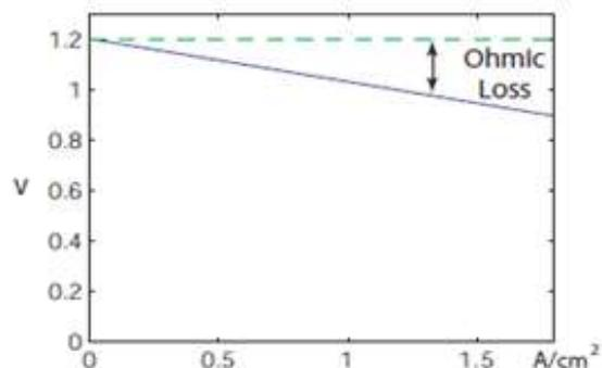
**Figure (3. 10):** The V-I characteristics of PEM Fuel Cell affected by the ohmic losses.
