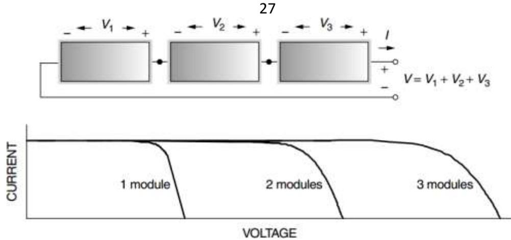
**Figure (3.3):** The I-V characteristics of 3 PV modules connected in series.
