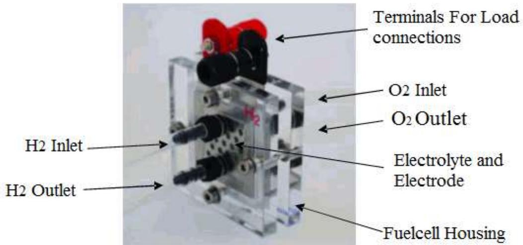
**Figure (4.8):** The PEM Fuel Cell.
