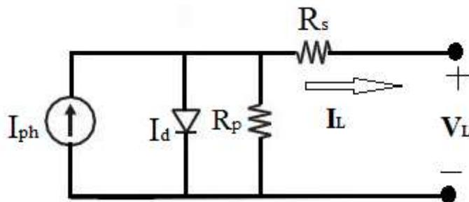
**Figure (3. 1):** Equivalent circuit of PV cell.
