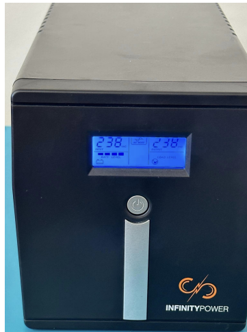
Figure 3.7: 800VA 480W UPS
