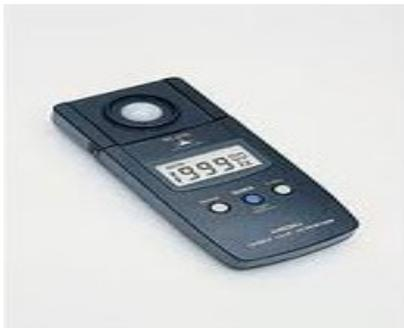
**Fig (2.1): Hioki 3424 lux Hitester Digital illumination**
