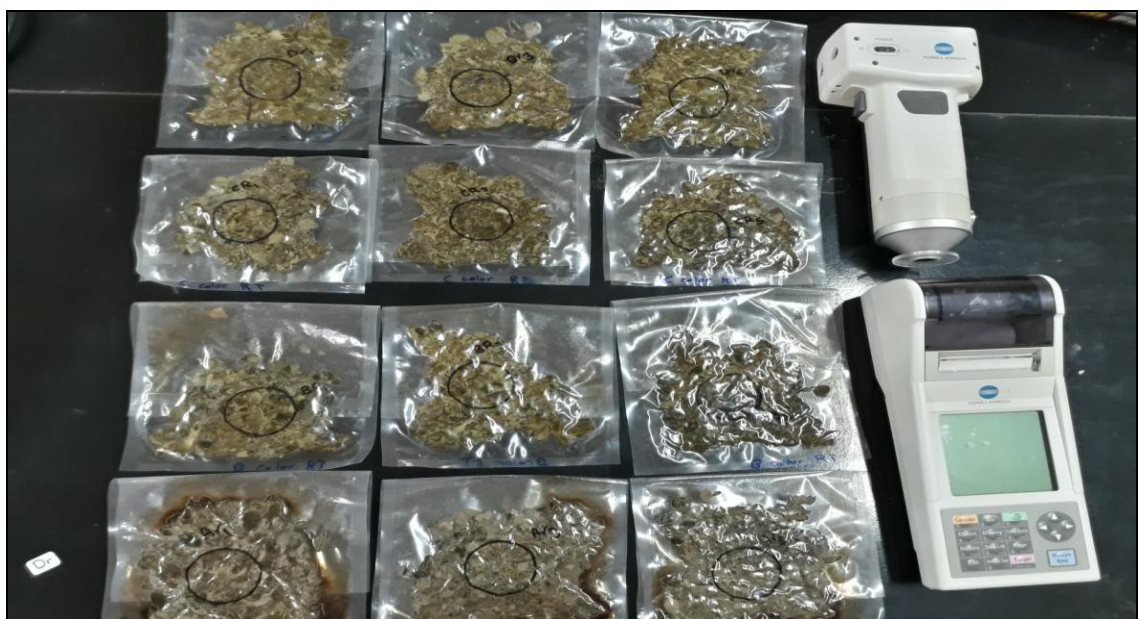
Image 2: Measurement of color indexes of green thyme samples by chromo meter
