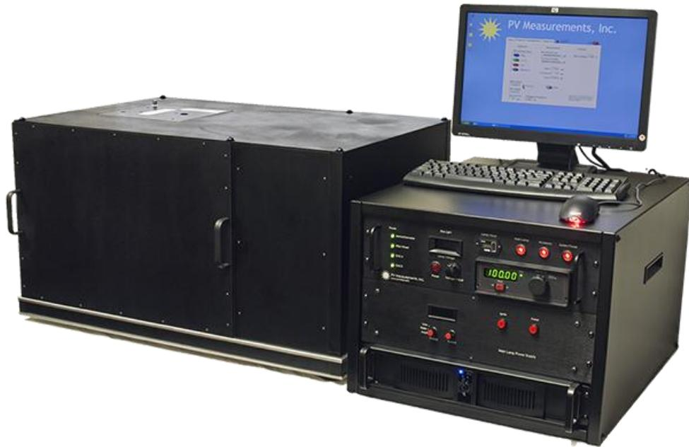
**Figure 3. 5:** QE monochromator-based setup.
