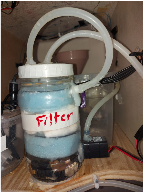
Figure 5.36: Water Filter Unit.
