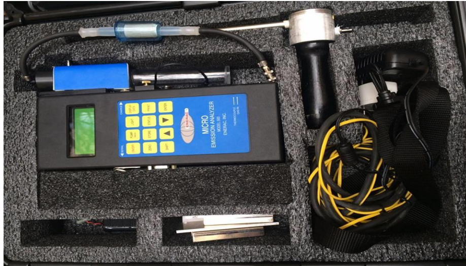
Figure 4.11 Combustion analyzer device
