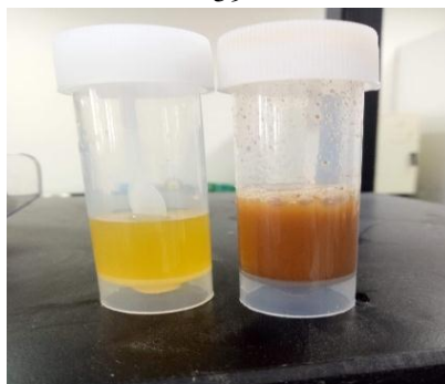
Figure 3.26: Images of waste water sample before and after treatment with the prepared polymer
