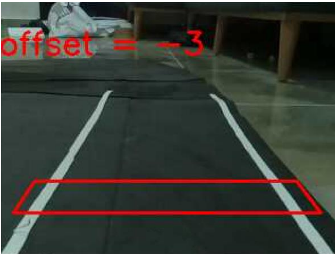
Figure 0-6-positioning lane and frame centers
